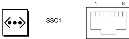
**FIGURE B-6** RJ-45 Twisted-Pair Ethernet Socket
