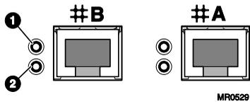
The LEDs to the left of each Ethernet connector indicate its status.
