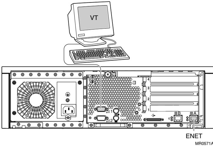
Figure 7–4 Setup for RMC with VGA Monitor
