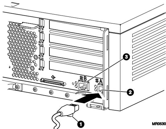
Connect the Ethernet cable ❶ to either Ethernet connector A ❷ or B ❸.
