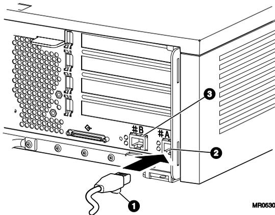
Connect the Ethernet cable **1** to either Ethernet connector A **2** or B **3**.
