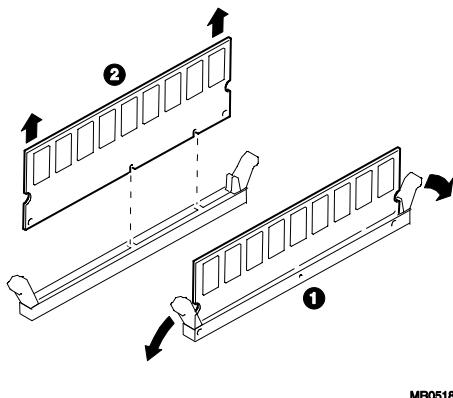
1. Release the clips ① securing the appropriate DIMM ②.
