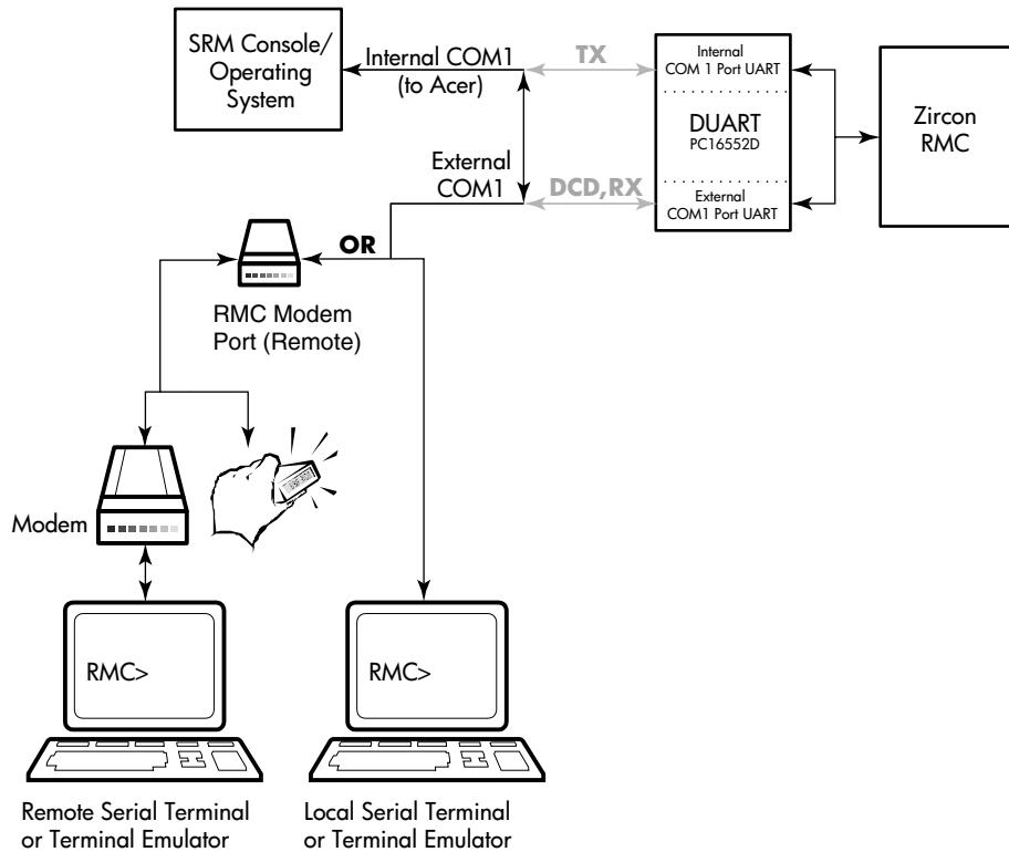
Figure 6–2 shows the data flow in the bypass modes. Note that the internal system COM1 port is connected directly to the external COM1 port.
