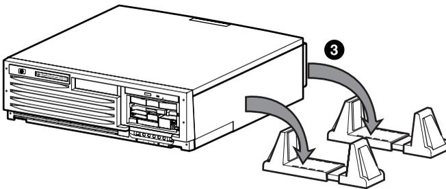
3. Close the supports securely against the system **4**. Pedestal systems must be positioned to allow proper airflow as shown in Figure 4-3.
