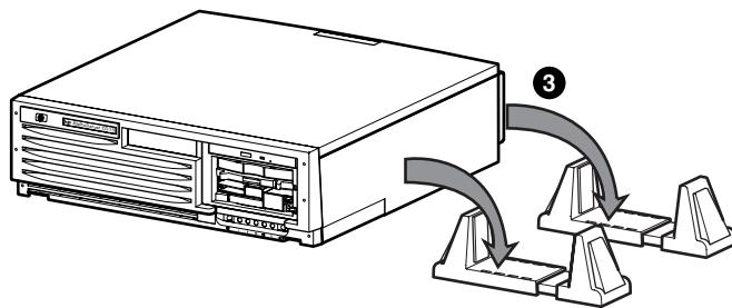
3. Close the supports securely against the system ④. Pedestal systems must be positioned to allow proper airflow as shown in Figure 4–3.
