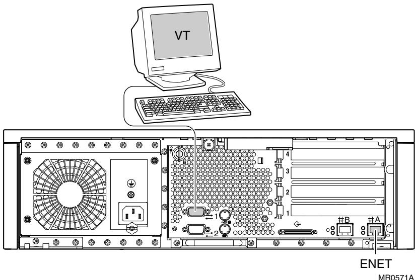
**Figure 6–4 Setup for RMC with VGA Monitor**
