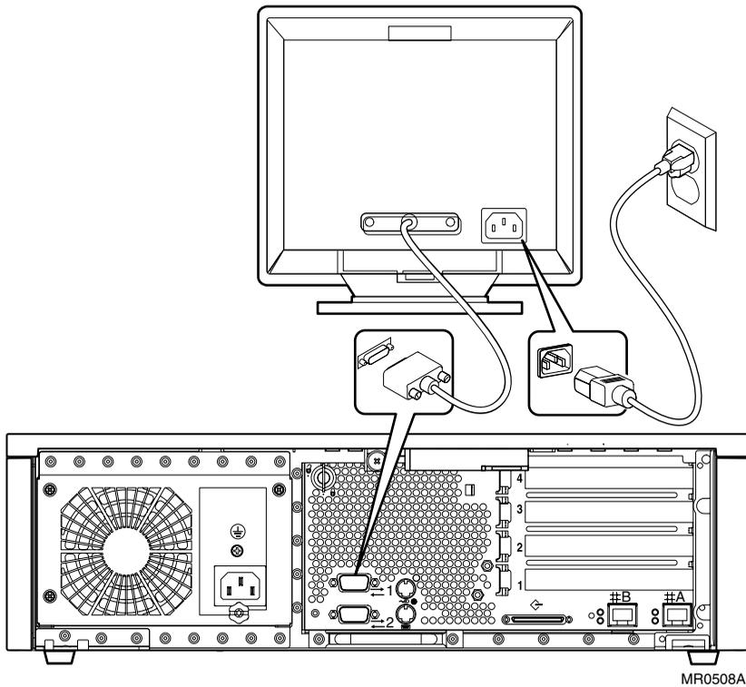
Figure 1-15 Console Terminal Connected to Optional Video Card
