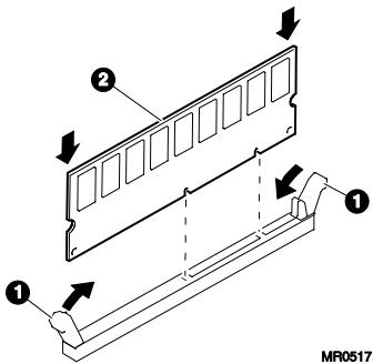
5. To install the DIMM ②, align the notches on the gold fingers with the connector keys as shown.
