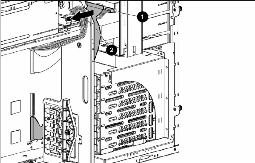
4. Remove the drive cage from the chassis.
