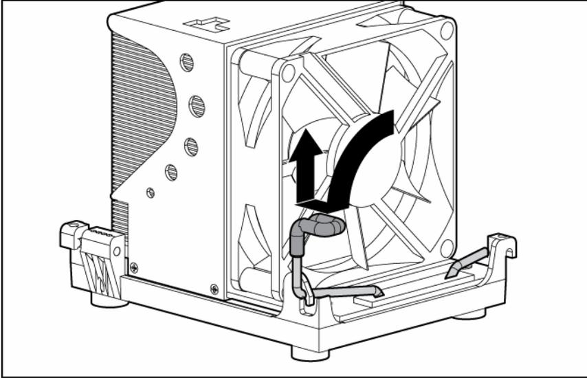
5. Connect the heatsink connector to the correct header on the system board.
