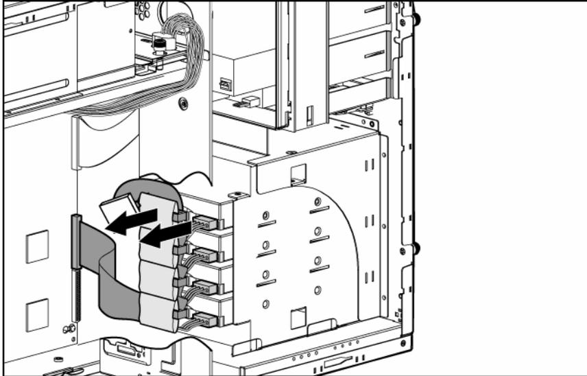
4. Remove screws from the hard drive bay, and remove the hard drive.
