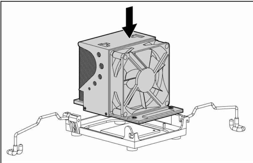
4. Close the processor retaining brackets.
