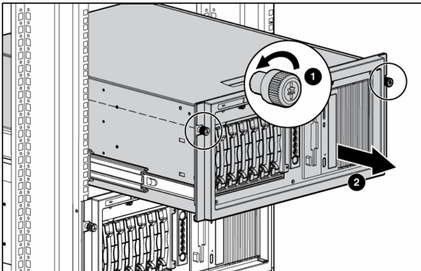
3. After performing the installation or maintenance procedure, slide the server back into the rack:
