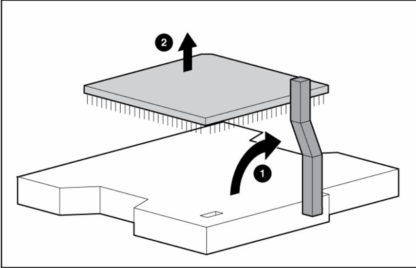
To replace the processor and heatsink:
