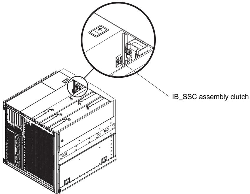
FIGURE 3-18 IB\_SSC Assembly Clutch Location
