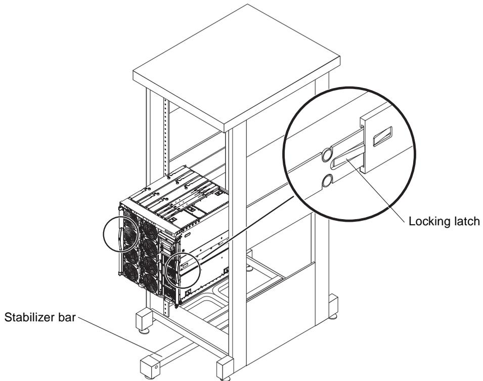
**FIGURE 2-5** Sliding the Server Out of the System Cabinet
