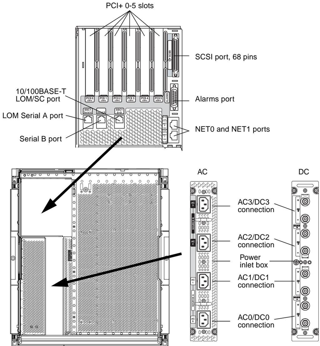
**FIGURE B-1** Netra 1290 Server External I/O Connections
