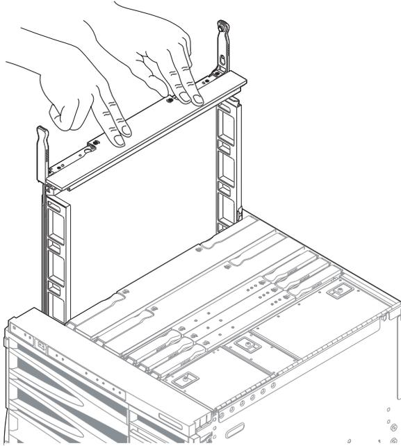
**FIGURE 5-1** Inserting a CPU/Memory Filler Board
