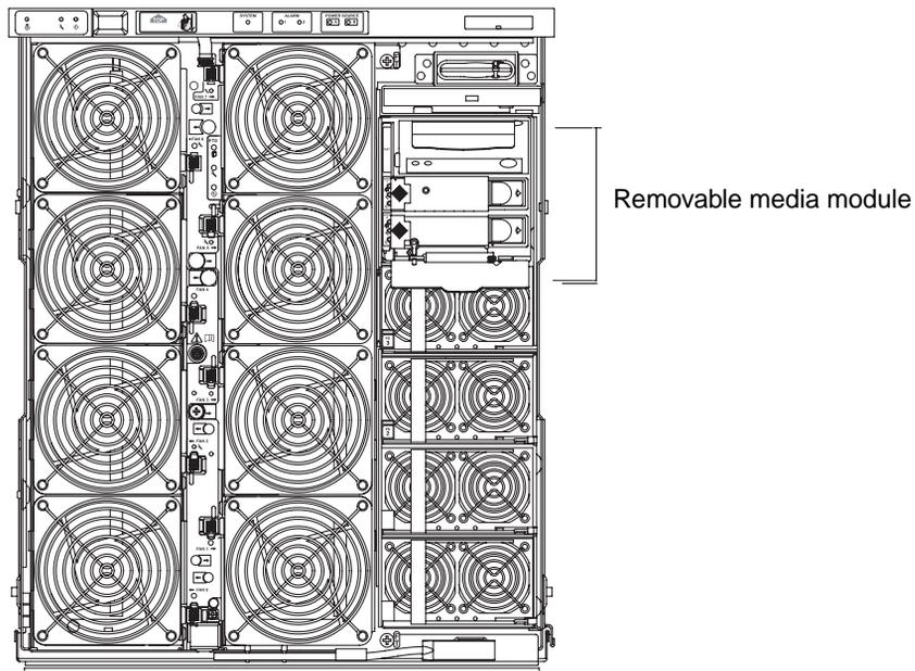
**FIGURE 4-5** Removable Media Module Location – Server Front View
