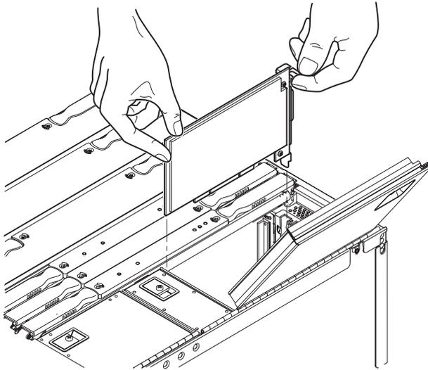
**FIGURE 5-24** Removing a I/O Card
