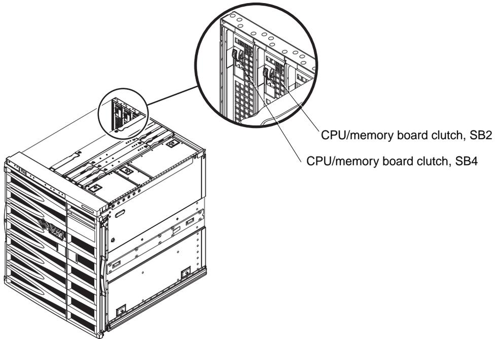
FIGURE 3-17 CPU/Memory Board Clutch Locations
