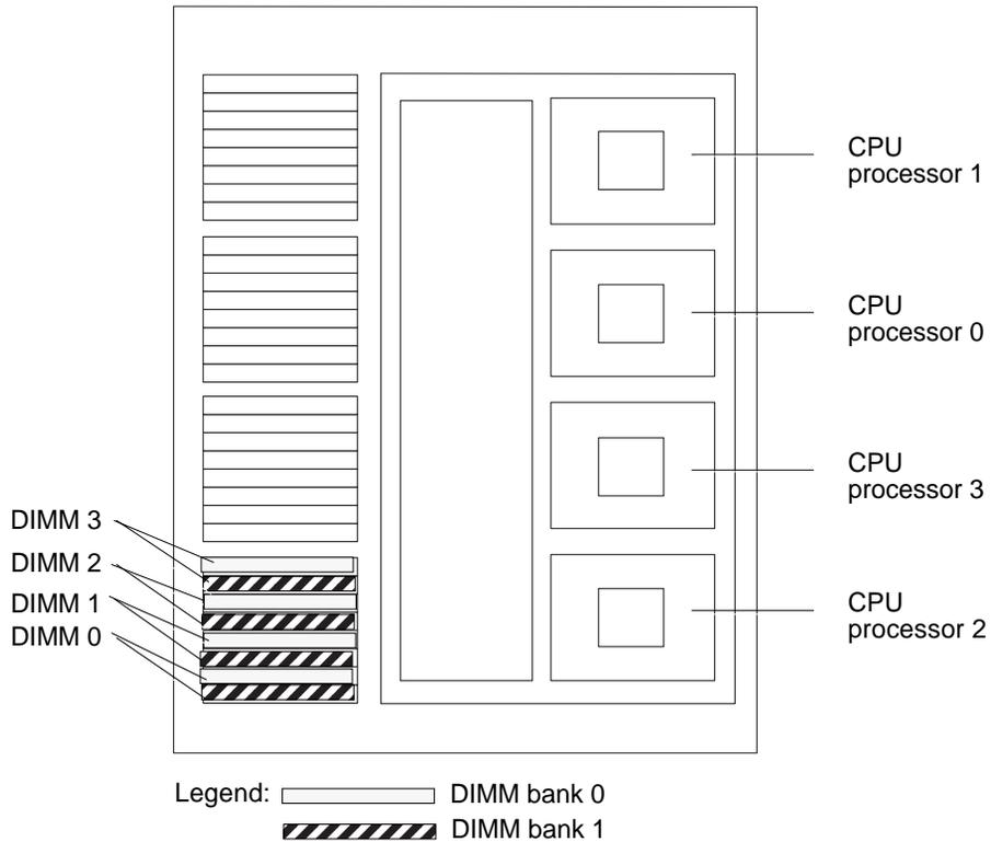
**FIGURE 5-9** DIMM Slot Numbers
