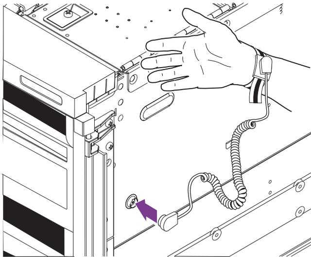
**FIGURE 2-1** Attaching the Antistatic Wrist Strap – Right Side
