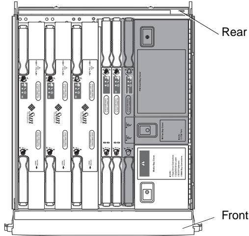
**FIGURE 5-16** IB\_SSC Assembly Location – Server Top View
