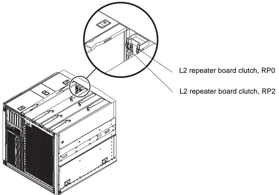
FIGURE 3-16 L2 Repeater Board Clutch Location
