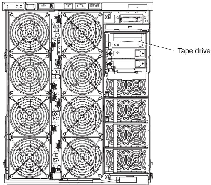
FIGURE 4-11 Tape Drive Location – Server Front View
