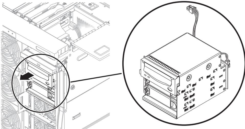
**FIGURE 4-9** Removing the Removable Media Module
