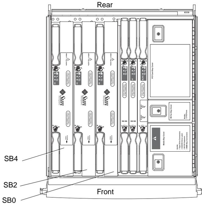
**FIGURE 5-2** Top View of the CPU/Memory Boards
