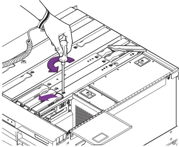
**FIGURE 5-19** Unlocking the IB\_SSC Assembly Ejector Levers
