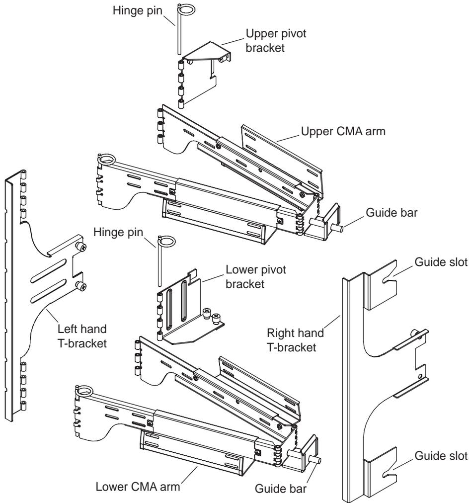
**FIGURE 3-3** Upper and Lower CMA Arms, and Left-Hand and Right-Hand T-Brackets
