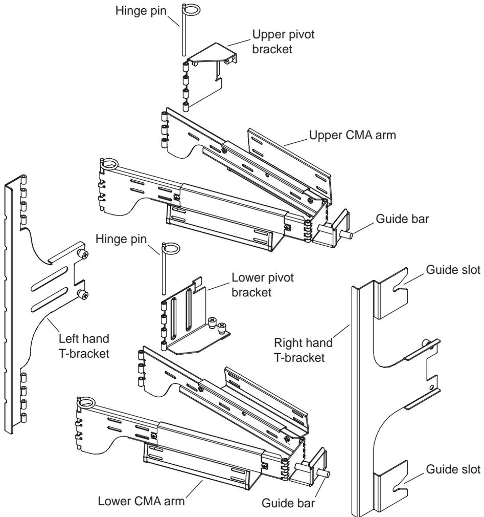
**FIGURE 3-9** Upper and Lower CMA Arms and Left-Hand and Right-Hand T-Brackets
