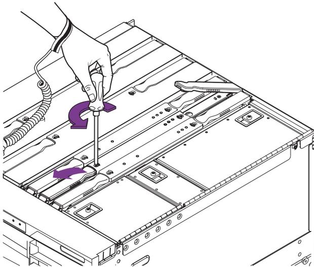
**FIGURE 5-14** Unlocking the L2 Repeater Board Ejector Levers
