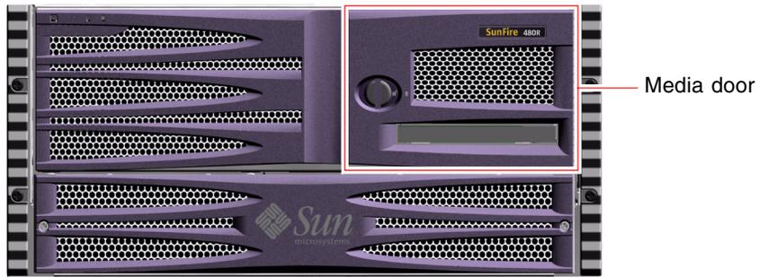
4. Insert the system key into the system control switch and turn the system control switch to the Normal position.
