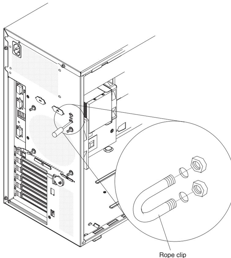
4. Thread the cable through the rope clip and around an object that is not part of or permanently secured to the building structure or foundation, and from which the cable cannot be removed. Fasten the cable ends together with a lock. After you add the security cable, make sure that it does not interfere with other cables that are connected to the server.
