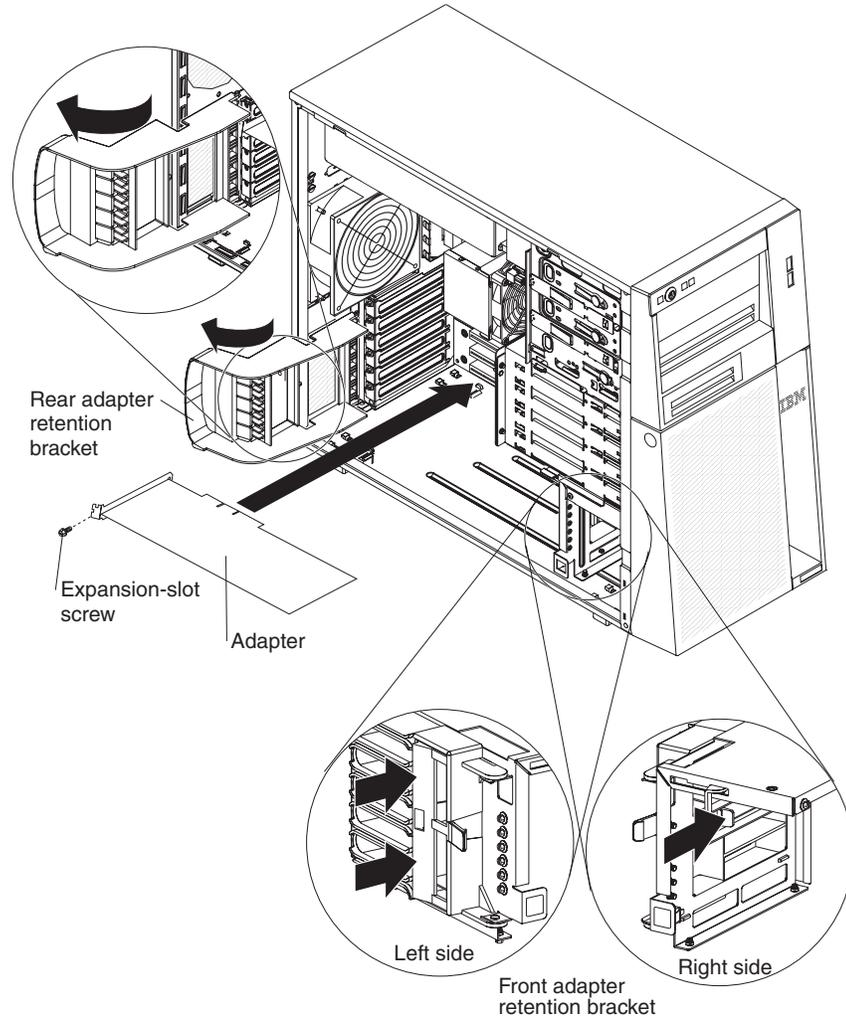
7. Touch the static-protective package that contains the adapter to any unpainted metal surface on the server. Then, remove the adapter from the static-protective package. Avoid touching the components and gold-edge connectors on the adapter.
