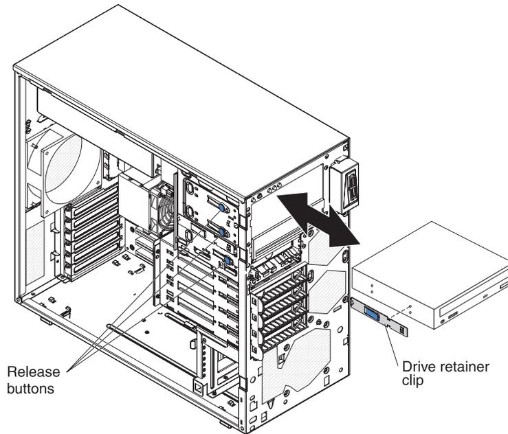
9. If you are installing a 5.2-inch drive in bay 2, slide the drive into the bay. If you are installing a 3.5-inch drive in bay 2, you must attach the 5.2-inch conversion kit to the 3.5-inch drive.
