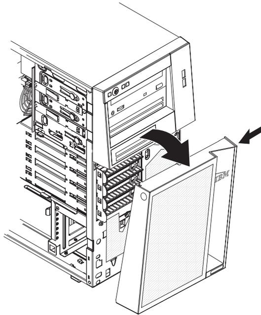
4. Lift the lower bezel to disengage the two bottom tabs from the chassis. Set the lower bezel aside.
