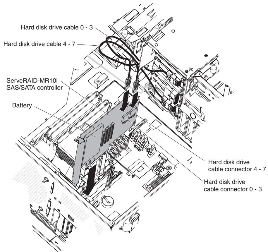
**Note:** The drive cage should be in the open position. This illustration shows it in the closed position.
