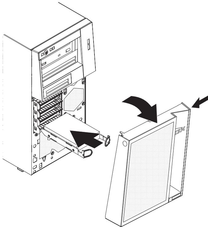
7. Pull the loops of the drive assembly toward each other; then, carefully slide the drive assembly into the drive bay until it stops, and release the loops.
