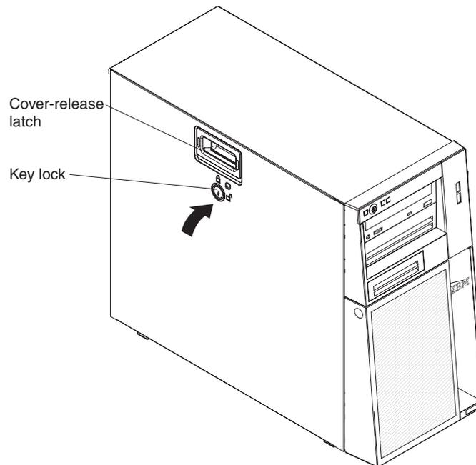
3. Close the cover-release latch to secure the side cover in place.
