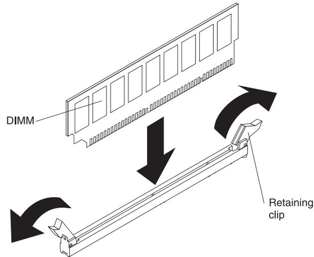
6. Touch the static-protective package that contains the DIMM to any unpainted metal surface on the server. Then, remove the new DIMM from the package.
