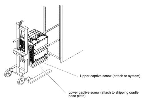
FIGURE 3-9 Securing the Captive Screws
