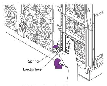
FIGURE 7-2 Unlatching a Power Supply
