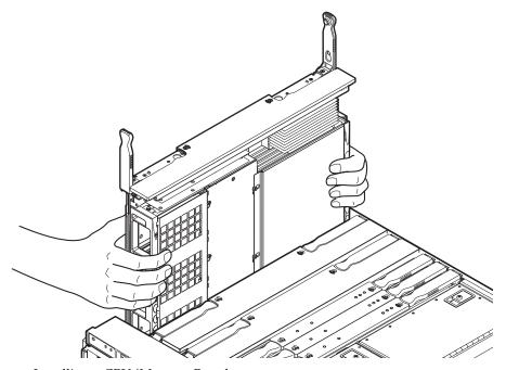
FIGURE 15-6 Installing a CPU/Memory Board
