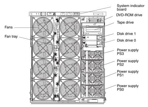
FIGURE 1-2 Front System View
