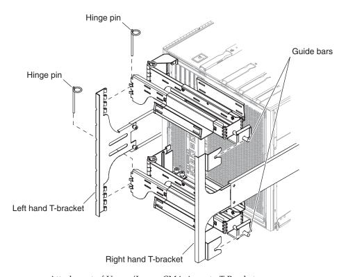
FIGURE 14-12 Attachment of Upper/Lower CMA Arms to T-Bracket
