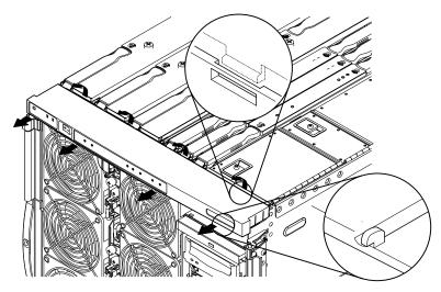
FIGURE 10-2 Removing the System Indicator Board Cover
