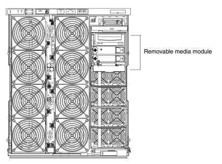
FIGURE 5-5 Removable Media Module Location—Front System View
