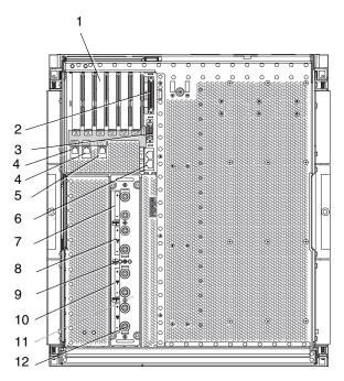
FIGURE 1-4 Rear View of the Netra 1280 System
