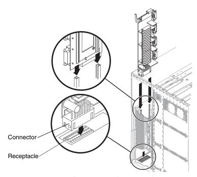
FIGURE 7-7 Inserting the Power Distribution Board
