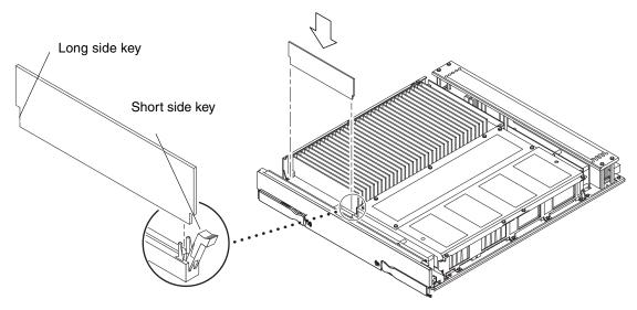
FIGURE 15-12 Installing a DIMM
