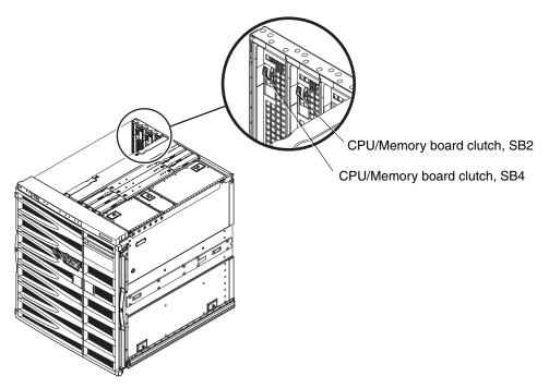
FIGURE 12-2 CPU/Memory Board Clutch Locations
