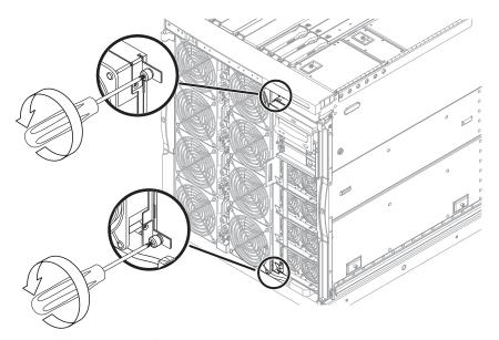
FIGURE 6-6 Loosening the Fan Tray Captive Screws
