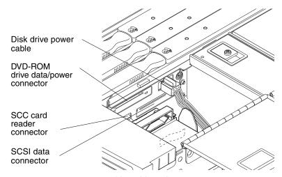
FIGURE 8-3 IB\_SSC Assembly Cable and Connector Locations
