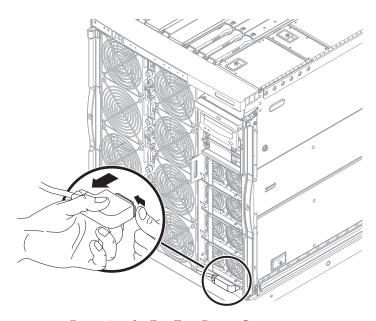
FIGURE 6-5 Removing the Fan Tray Power Connector
