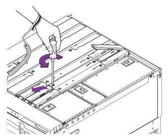
FIGURE 9-2 Unlocking the L2 Repeater Board Ejector Levers
