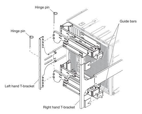
FIGURE 14-4 Detachment of Upper/Lower CMA Arms to T-Bracket
