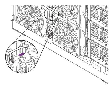
FIGURE 6-1 Disconnecting the Fan Power Connector
