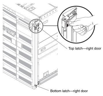
FIGURE 2-4 Releasing the Front Door Latches
