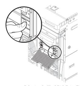
FIGURE 5-2 Releasing the Hard Disk Drive Ejector
