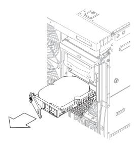
FIGURE 5-4 Removing the Hard Disk Drive
