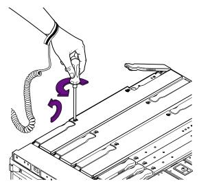
FIGURE 15-3 Unlocking the CPU/Memory Board Ejector Levers
