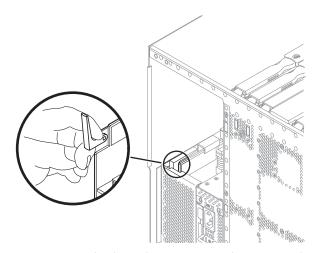
FIGURE 7-5 Unlatching the Power Distribution Board Ejector Lever
