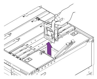
FIGURE 6-11 Removing an IB\_SSC Fan
