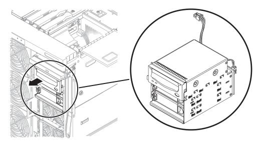
FIGURE 5-10 Removing the Removable Media Module
