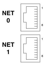
FIGURE B-3 RJ-45 Gigabit Ethernet Connectors
