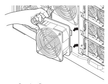
FIGURE 6-3 Removing a Fan
