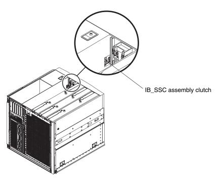
FIGURE 12-3 IB\_SSC Assembly Clutch Location
