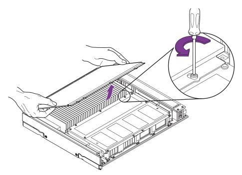
FIGURE 15-10 Removing the DIMM Cover
