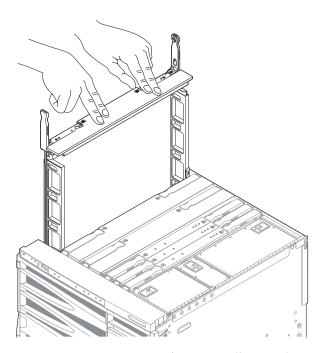
FIGURE 15-1 Inserting a CPU/Memory Filler Board
