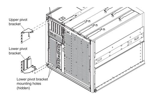
FIGURE 14-7 Upper/Lower Pivot Bracket Mounting Holes
