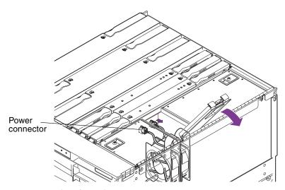
FIGURE 6-10 Identifying the Fan Power Connector
