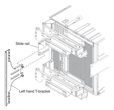
FIGURE 14-5 Detaching Left Hand T-Bracket
