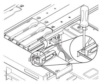
FIGURE 5-23 Loosening the SCC Reader Captive Screw
