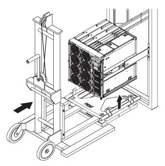
FIGURE 3-8 Lifting Device and Shipping Cradle
