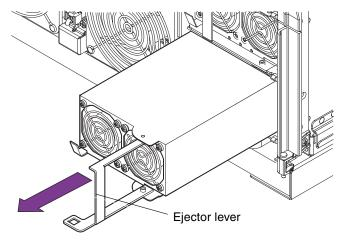
FIGURE 7-3 Removing a Power Supply
