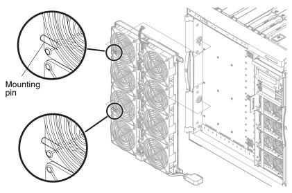
**FIGURE 6-7** Removing the Fan Tray
