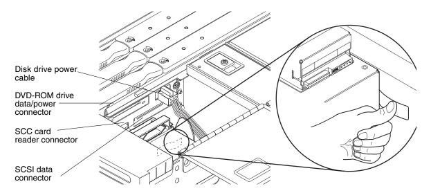
FIGURE 5-7 IB\_SSC Assembly Cable and Connector Locations
