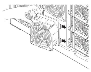
**FIGURE 6-4** Inserting a Fan into the Fan Tray
