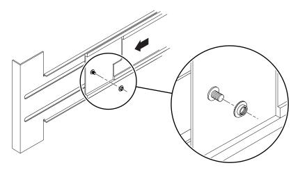
FIGURE 3-11 Inserting and Tightening the Spacer
