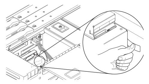
FIGURE 5-8 Releasing the Removable Media Module Retaining Spring
