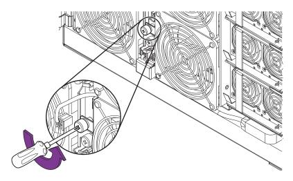
FIGURE 6-2 Loosening the Fan's Captive Screw
