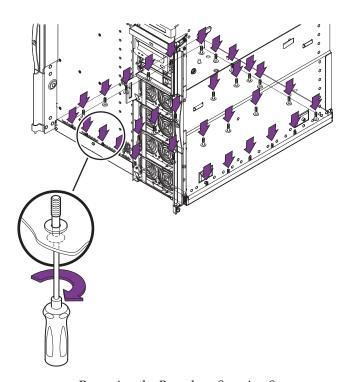
FIGURE 11-2 Removing the Baseplane Securing Screws
