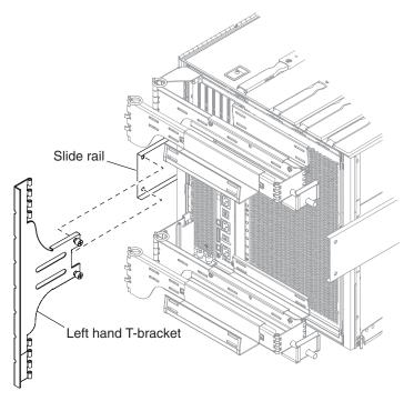
FIGURE 14-10 Attaching Left Hand T-Bracket
