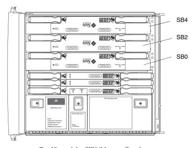
FIGURE 15-2 Top View of the CPU/Memory Boards
