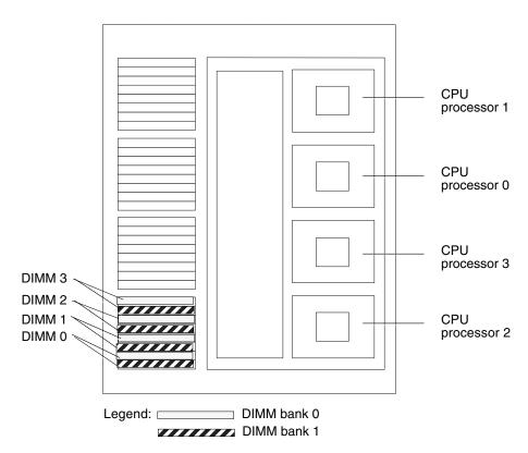
FIGURE 15-9 DIMM Slot Numbers
