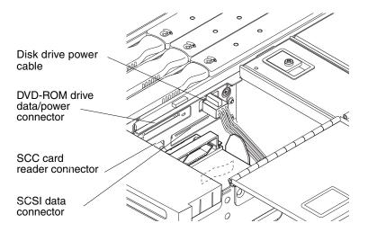
FIGURE 5-18 IB\_SSC Assembly Cable and Connector Locations
