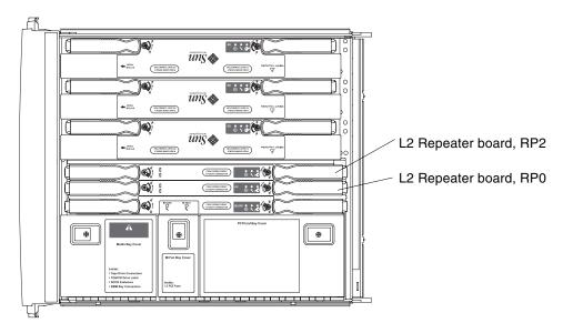
FIGURE 9-1 Location of Boards, Modules, and Bays—System Top View
