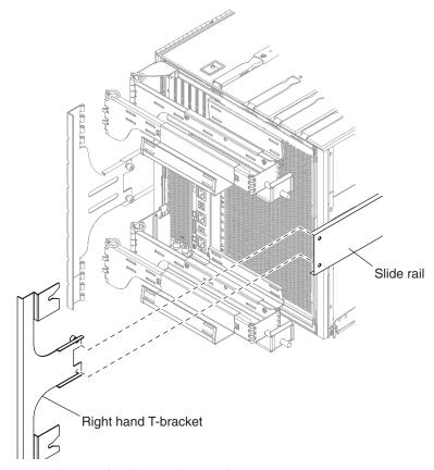
FIGURE 14-11 Attachment of Right-Hand T-Bracket
