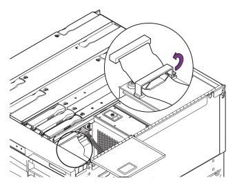
FIGURE 5-21 Disconnecting the IDE Cable
