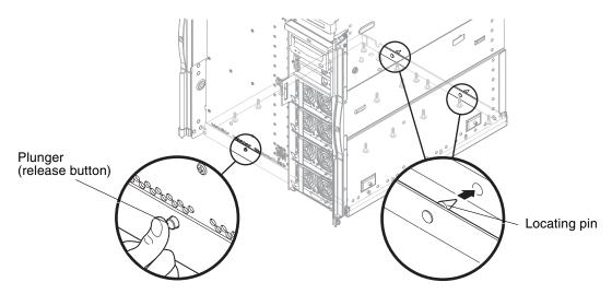
FIGURE 11-3 Releasing the Baseplane Plunger (If Fitted)
