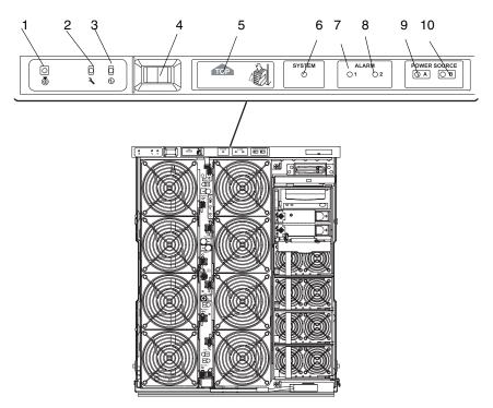
FIGURE 1-5 System Front Panel LEDs
