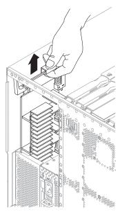
FIGURE 7-6 Removing the Power Distribution Board
