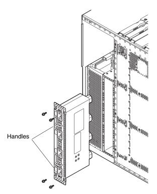
FIGURE 7-4 Removing the Power Inlet Box (Sun Fire V1280 Shown)
