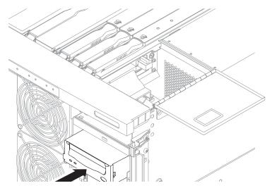
FIGURE 5-15 Inserting a Tape Drive into the System
