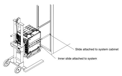
FIGURE 3-10 Detaching the Cabinet Slides From the System
