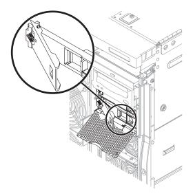
FIGURE 5-3 Ejecting the Hard Disk Drive
