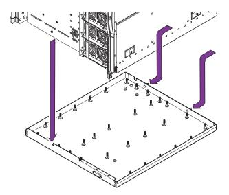
FIGURE 11-4 Removing the Baseplane
