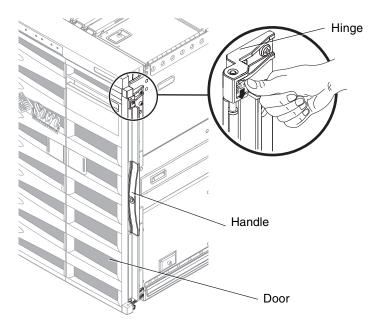
FIGURE 13-1 Bezel Hinge Release Mechanism
