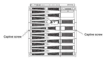
FIGURE 3-3 Side Handle Captive Screws
