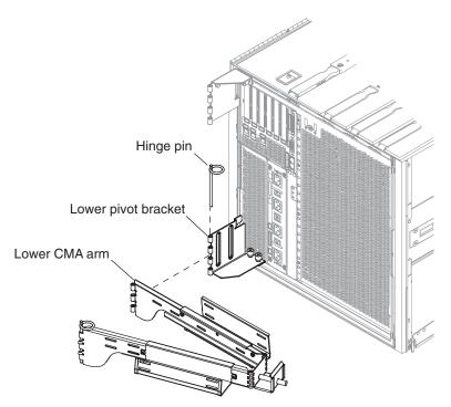
FIGURE 14-9 Attachment of Lower CMA Arm and Pivot Bracket
