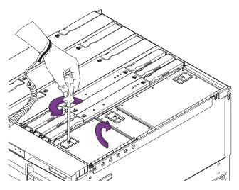
FIGURE 8-2 Opening the Media Bay Cover—System Top View
