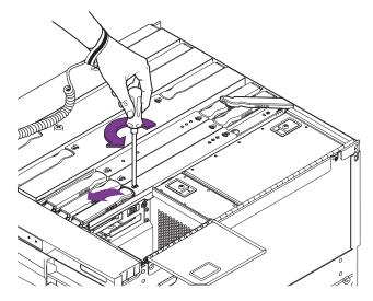
FIGURE 8-4 Unlocking the IB\_SSC Assembly Ejector Levers
