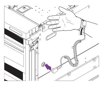
FIGURE 2-2 Attaching the Antistatic Wrist Strap—Right Side
