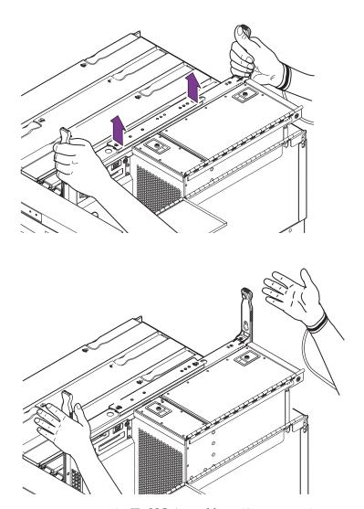
FIGURE 8-5 Raising the IB\_SSC Assembly Halfway Using the Antigravity Guides
