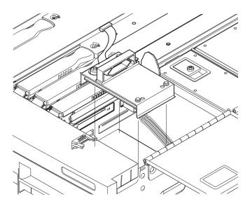
FIGURE 5-24 Removing the SCC Reader
