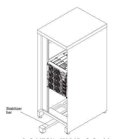
FIGURE 2-1 Sun Rack 900 Cabinet With Stabilizer Bar Extended
