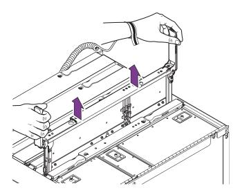
FIGURE 9-3 Raising an L2 Repeater Board
