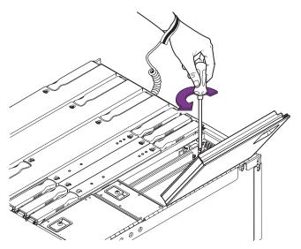
FIGURE 8-8 Removing the I/O Card Retaining Screw
