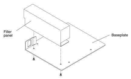
FIGURE 5-13 Dismantling the Tape Drive Filler Panel
