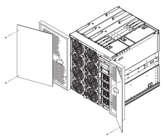
FIGURE 2-6 Installing the Sun Fire V1280/Netra 1280 System Air Filters
