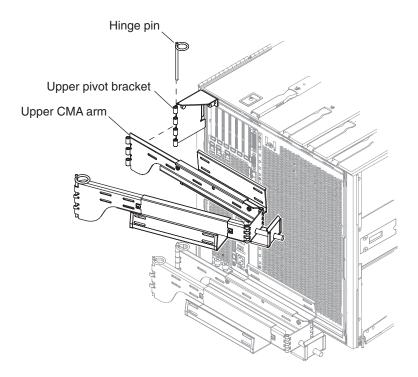
FIGURE 14-8 Attachment of Upper CMA Arm and Pivot Bracket
