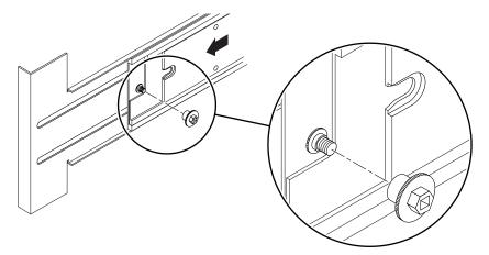
FIGURE 3-12 Inserting and Tightening the Locking Nut
