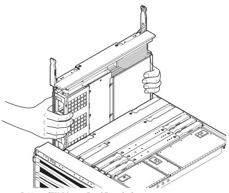
FIGURE 15-5 Raising a CPU/Memory Board From the System
