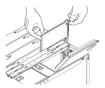
FIGURE 8-9 Removing a I/O Card
