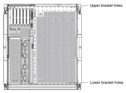
FIGURE 14-1 Bracket Mounting Holes
