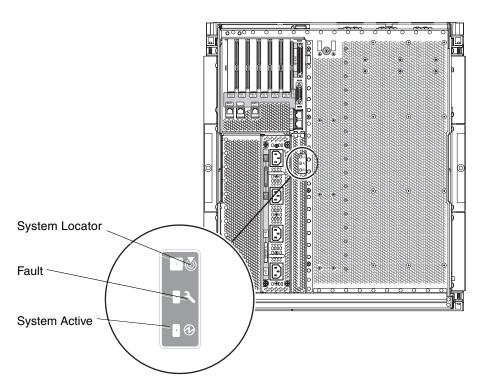
FIGURE 1-6 System LEDs on the Rear Panel
