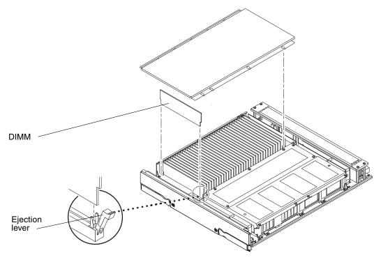
FIGURE 15-11 Removing a DIMM
