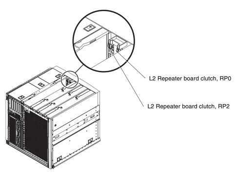
FIGURE 12-1 L2 Repeater Board Clutch Location
