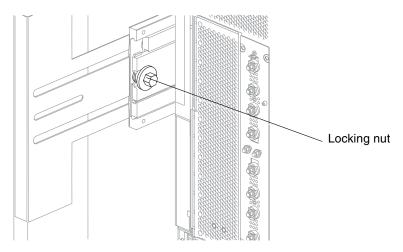
FIGURE 3-4 Slide Locking Nut
