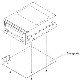
FIGURE 5-14 Assembling the Tape Drive
