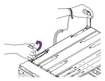
FIGURE 15-4 Raising the CPU/Memory Board Ejector Levers
