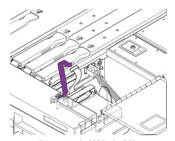
FIGURE 5-22 Disconnecting the SCC Reader Cable
