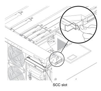
FIGURE 5-20 System Configuration Card Slot Location
