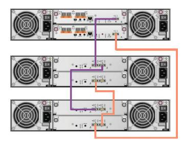
Figure 20. Reverse cabling example using the MSA 2050 system
