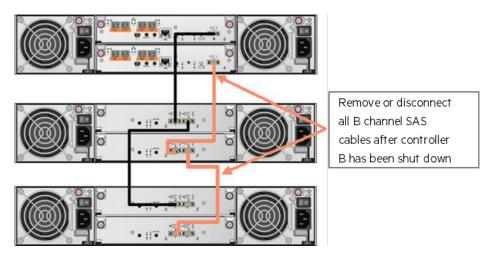
Figure 28. Straight-through cabling configuration
