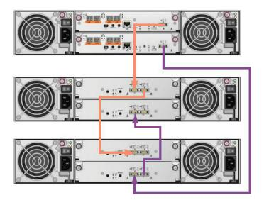
Figure 26. Fault-tolerant cabling configuration
