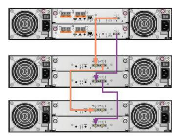
Figure 25. Straight-through cabling configuration
