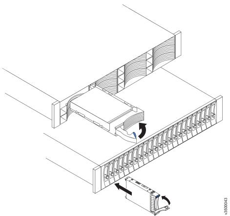
Figure 25. Installing a drive
