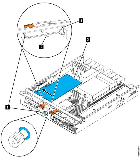
Figure 17. Installing 10 Gbps iSCSI-FCoE 2 port host interface card
