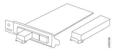
Figure 15. Host interface card and SFP transceivers
