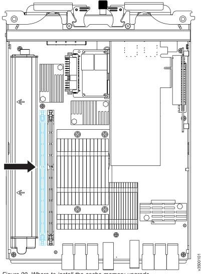
Figure 20. Where to install the cache memory upgrade
