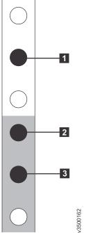
Figure 9. Hole locations in the front of the rack
