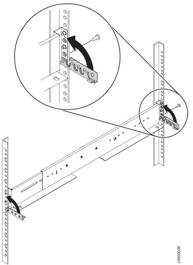
Figure 11. Closing hinge brackets and installing rear screw
