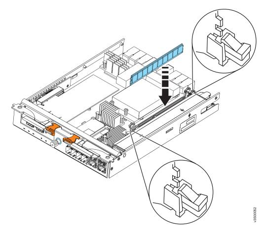
Figure 21. Installing memory module option
