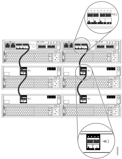
Figure 27. Connecting the SAS cables
