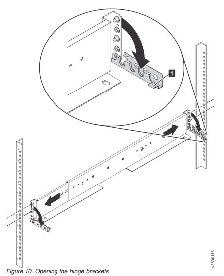
6. Align the holes in the rail bracket with the holes on the front and rear rack cabinet flanges. Ensure that the rails are aligned on the inside of the rack cabinet.
