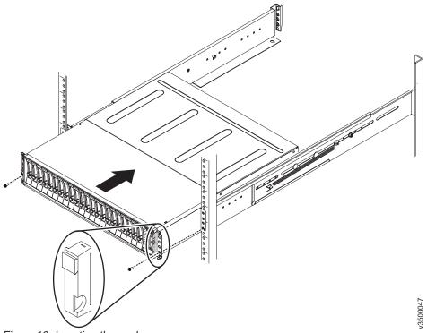
Figure 12. Inserting the enclosure
