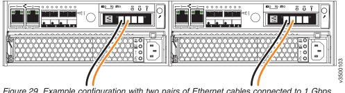
Figure 29. Example configuration with two pairs of Ethernet cables connected to 1 Gbps iSCSI 4-port host interface cards
