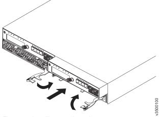
Figure 23. Installing a node canister
