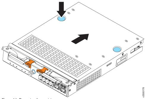
Figure 14. Removing the canister cover
