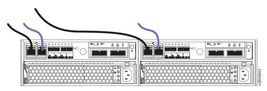
Figure 28. Connecting the Ethernet cables
