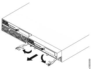
Figure 13. Removing a node canister
