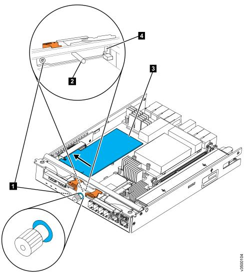
Figure 19. Installing SAS 4-port host interface card
