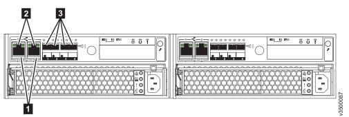
Figure 2. Data ports in the rear of the control enclosure
