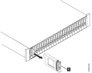
Figure 24. Removing a filler panel
