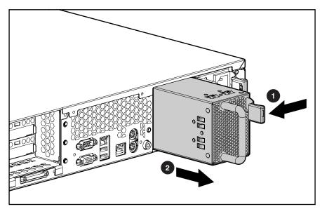
Figure 2-10. Removing the power supply blank
