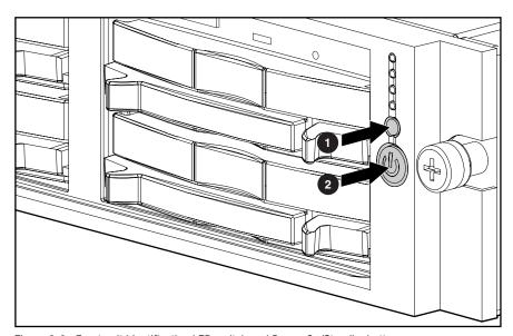
Figure 2-2. Front unit identification LED switch and Power On/Standby button
