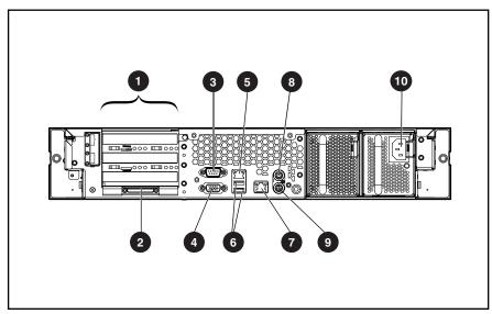
Figure 4-1. Rear panel connectors
