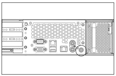
Figure 4-8. Rear unit identification LED switch
