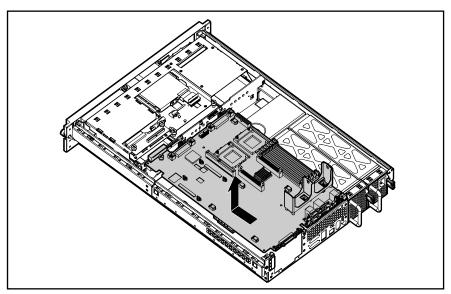
Figure 2-54. Removing the system board from the chassis
