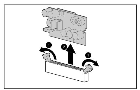
Figure 2-49. Removing a PPM
