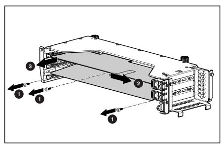
Figure 2-35. Removing the PCI expansion board ejector/divider
