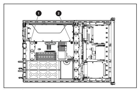
Figure 4-5. PCI riser cage LEDs
