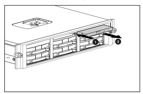
Figure 2-24. Ejecting the CD-ROM drive
