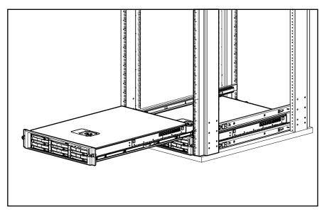
Figure 2-1. Extending the server from the rack
