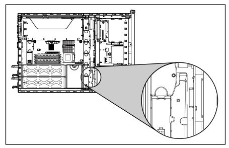
Figure 4-11. Power converter module LED
