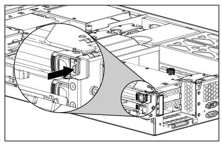
Figure 2-19. Pressing the PCI Hot Plug button
