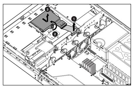
Figure 2-25. Removing the diskette drive
