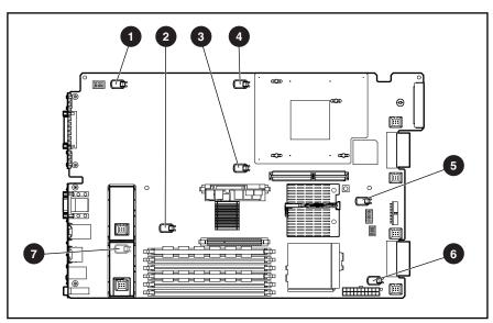
Figure 2-53. Identifying the alignment keys and keyhole locations
