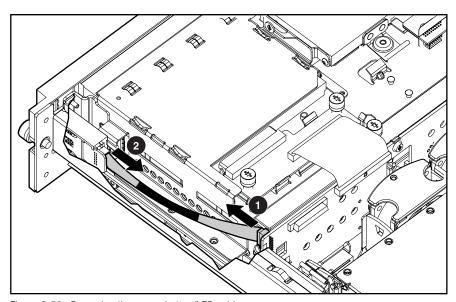
Figure 2-58. Removing the power button/LED cable
