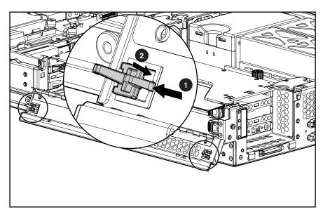
Figure 2-17. Removing the PCI riser cage door latch
