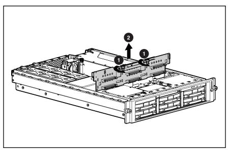
Figure 2-30. Removing the SCSI backplane
