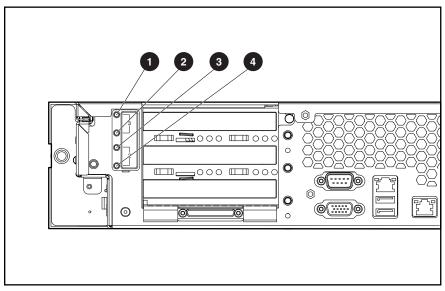
Figure 4-6. PCI Hot Plug button LEDs
