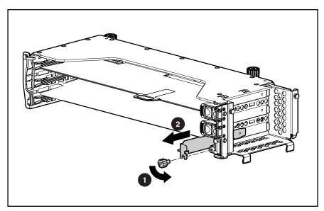
Figure 2-34. Removing the expansion slot cover from slot 1
