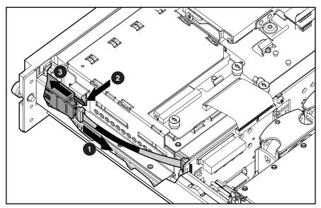
Figure 2-42. Removing the power button/LED board
