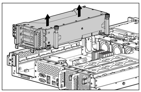
Figure 2-32. Removing the PCI riser cage
