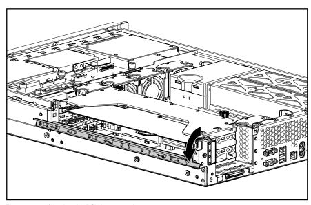
Figure 2-18. Opening the PCI riser cage door
