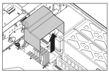
Figure 2-14. Removing the air baffle
