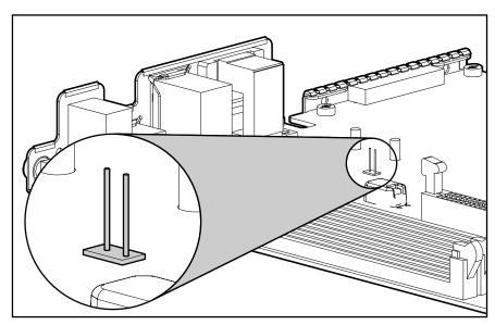
Figure 4-14. Bootblock flash jumper
