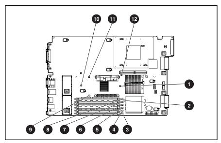
Figure 4-12. System board LEDs
