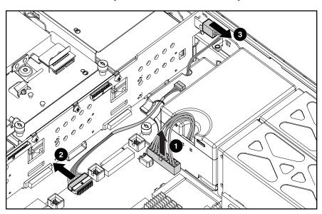
Figure 2-40. Disconnecting the power cables
