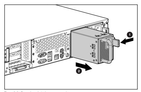
Figure 2-9. Removing a hot-plug power supply
