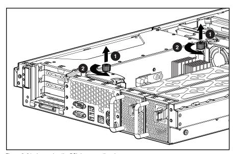
Figure 2-31. Loosening the PCI riser cage thumbscrews
