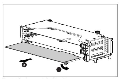
Figure 2-33. Removing an expansion board from slot 1
