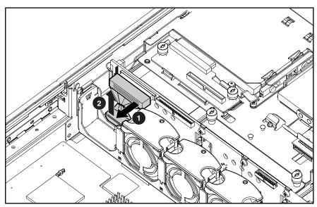
Figure 2-56. Removing the short SCSI cable (PCI riser cage removed for clarity)
