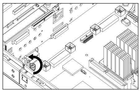
Figure 2-52. Loosening the system board thumbscrew
