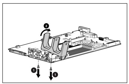
Figure 2-55. Removing the rear fan bracket
