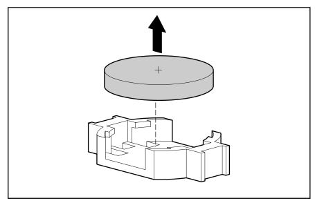
Figure 2-51. Removing the battery
