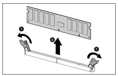
Figure 2-43. Removing a DIMM
