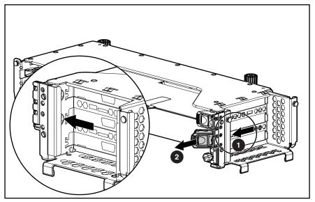
Figure 2-37. Removing the PCI slot release lever
