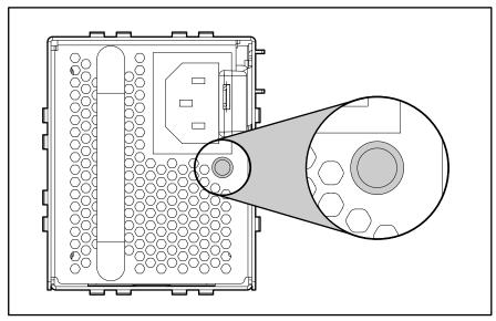
Figure 4-9. Hot-plug power supply LED
