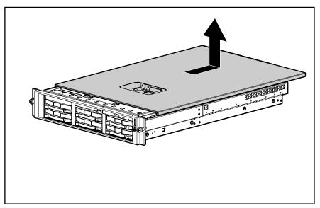
Figure 2-12. Removing the access panel
