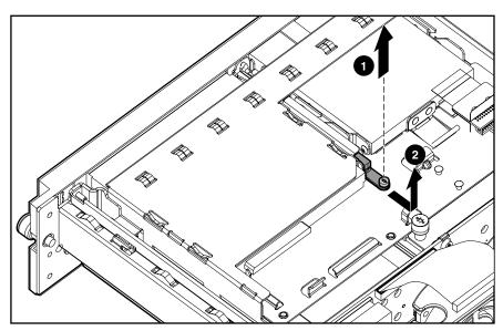
Figure 2-28. Removing the CD ejector assembly
