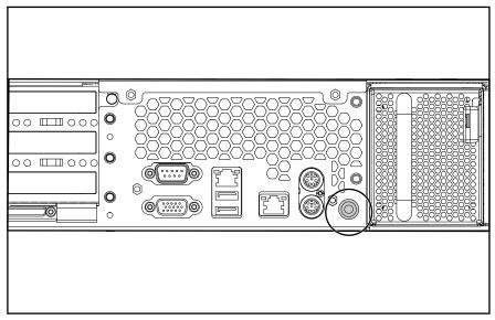
Figure 2-3. Rear unit identification LED switch
