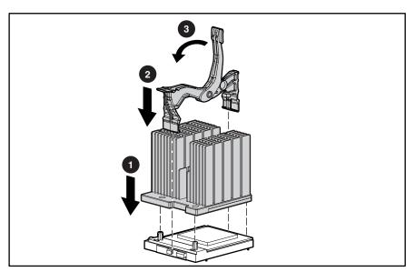
Figure 2-48. Installing the heatsink and heatsink-retaining clip
