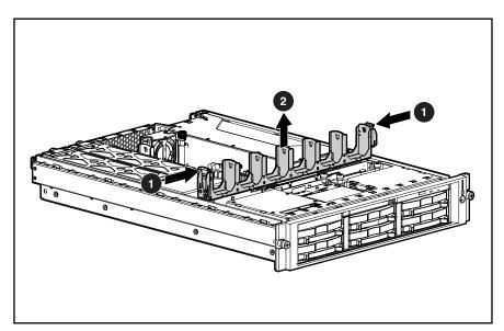
Figure 2-29. Removing the front fan bracket
