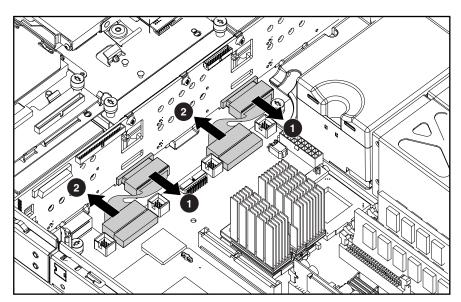
Figure 2-59. Removing the system cables (PCI riser cage removed for clarity)
