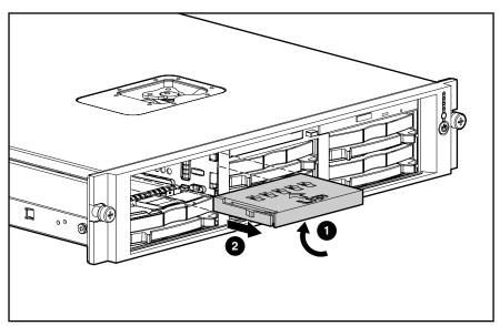
Figure 2-8. Removing the tape drive blank
