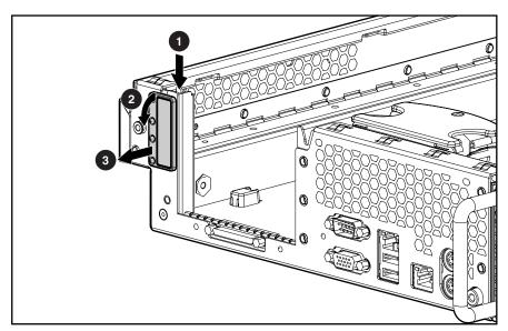
Figure 2-38. Removing the PCI lightpipe cover
