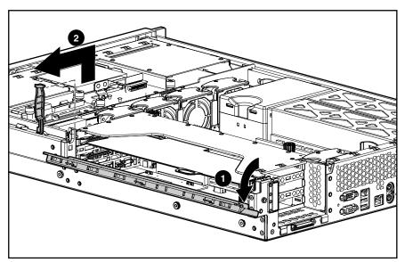
Figure 2-15. Removing the PCI shipping bracket
