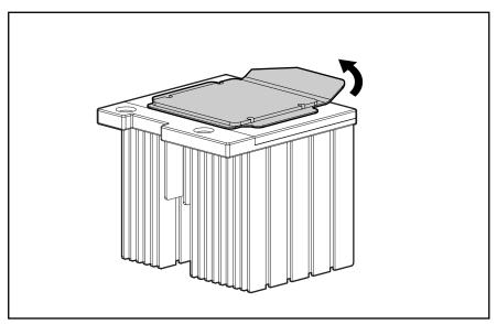
Figure 2-47. Removing the plastic strip on the heatsink
