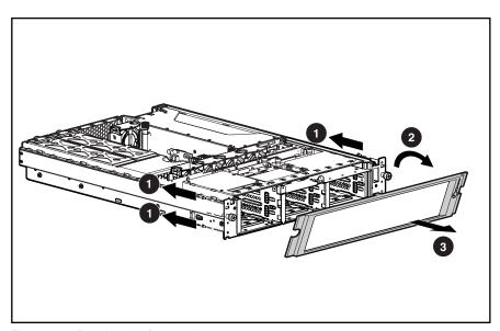
Figure 2-23. Removing the front bezel
