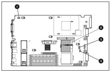
Figure 4-13. System board switches
