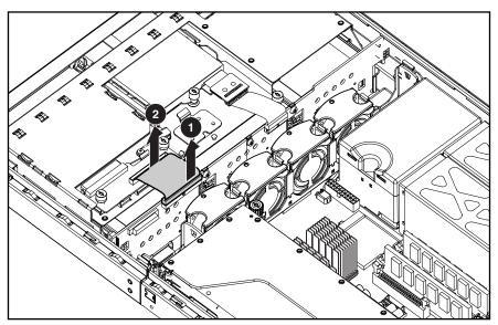
Figure 2-57. Removing the CD MultiBay cable
