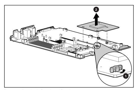
Figure 2-50. Removing the Smart Array 5i Controller
