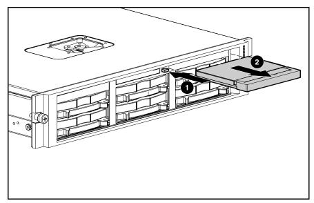
Figure 2-6. Removing the CD blank
