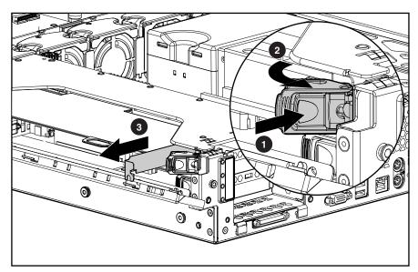
Figure 2-22. Removing the expansion slot cover from slot 3
