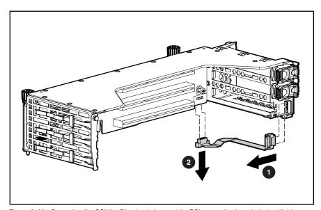
Figure 2-60. Removing the PCI Hot Plug backplane cable (PCI expansion board ejector/divider removed for clarity)
