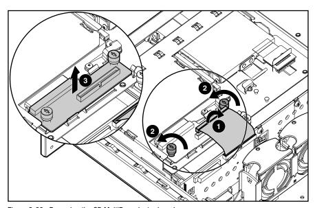
Figure 2-26. Removing the CD MultiBay adapter board
