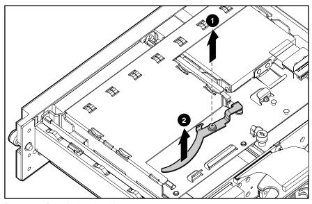
Figure 2-27. Removing the ejector lever
