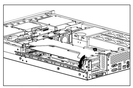
Figure 2-21. Opening the PCI riser cage door
