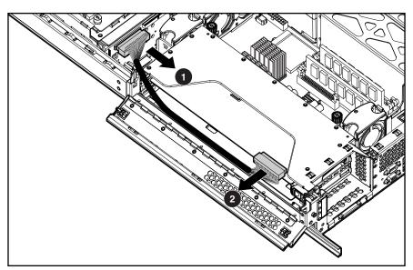
Figure 2-62. Removing the long SCSI cable
