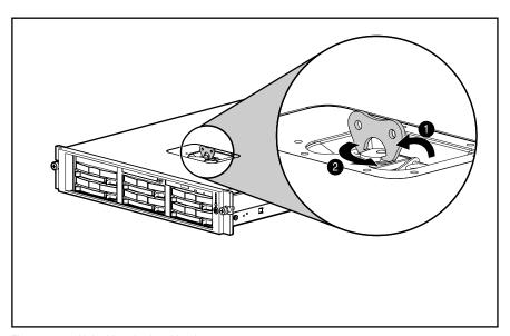
Figure 2-11. Unlocking the hood latch
