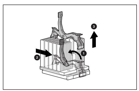
Figure 2-44. Disengaging the heatsink-retaining clip
