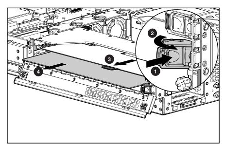
Figure 2-20. Removing an expansion board from slots 2 and 3
