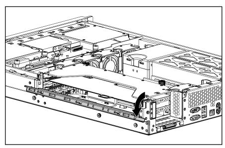
Figure 2-16. Opening the PCI riser cage door
