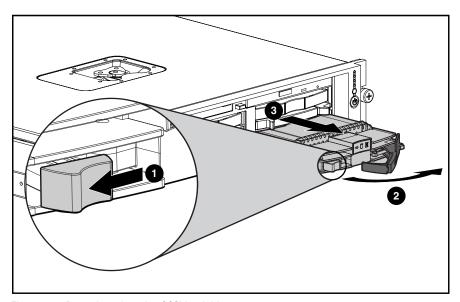
Figure 2-4. Removing a hot-plug SCSI hard drive
