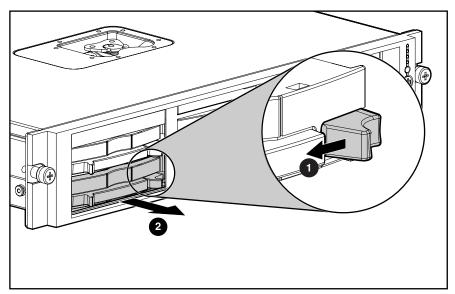
Figure 2-5. Removing a hard drive blank
