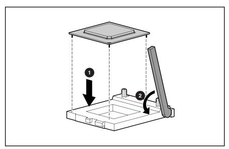
Figure 2-46. Installing the processor
