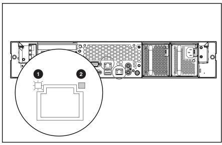
Figure 4-7. RJ-45 network connector LEDs
