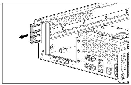
Figure 2-39. Sliding the lightpipe out of the chassis
