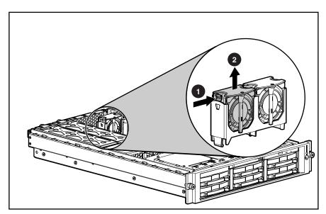
Figure 2-13. Removing a fan
