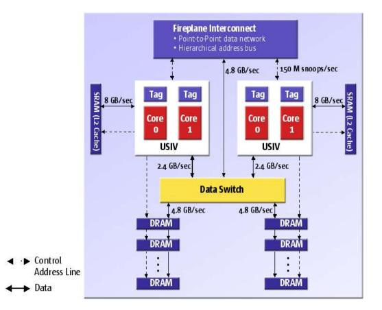
Figure 3-5: UltraSPARC IV System interface
