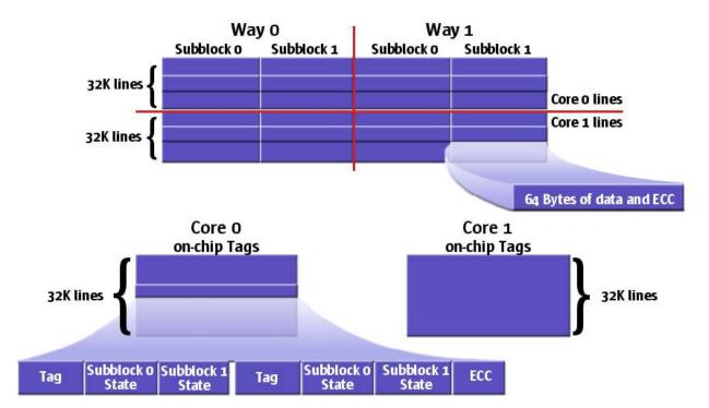
Figure 3-4: UltraSPARC IV Level 2 cache structure
