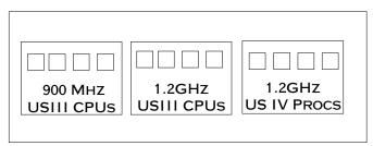
• The diagram below illustrates the three-step upgrade process to upgrade all CPUs on two CPU/memory boards. During this online upgrade process, the application remains available.
