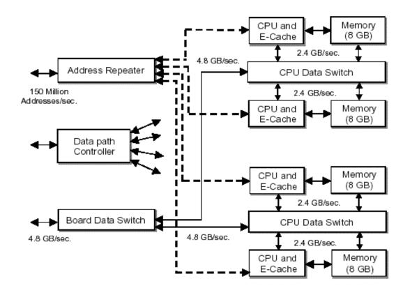
Figure 4-2: CPU/memory board block diagram
