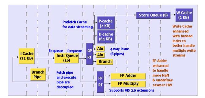
Figure 3-3: UltraSPARC IV execution pipeline
