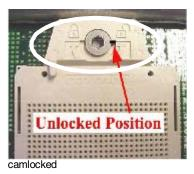
When installing the CPU module, use care to insert all processor pins into the socket simultaneously. The two connectors must be parallel as the pins are inserted in to the sockets.
