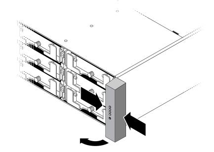
FIGURE 5-1 Removing the Right Ear Cap
