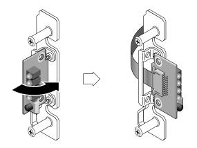
FIGURE 5-3 Removing the LED Module
