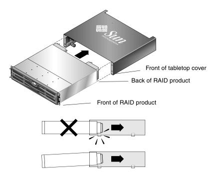
FIGURE 2-6 Sliding the Chassis Into the Tabletop Cover
