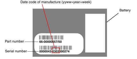
FIGURE 4-2 Battery Label Example for the Sun StorEdge 3510 FC Array
