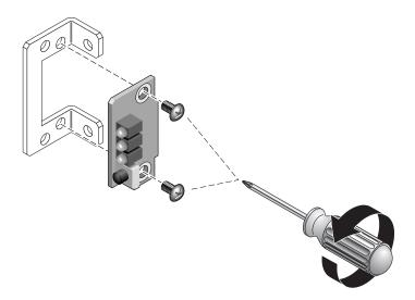
FIGURE 5-12 Detaching the LED Module From the Bracket
