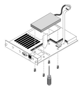
FIGURE 4-7 The Top and Side View of the Controller Module With the Battery Being Inserted
