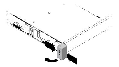
FIGURE 5-7 Removing the Right Ear Cap
