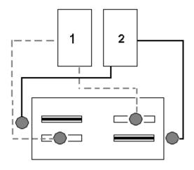
FIGURE 10-3 Two Terminators for Two Cables That Have Been Removed in a Split-Bus Configuration
