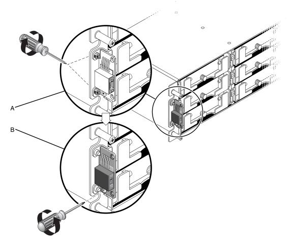
FIGURE 9-10 Detaching the ID Switch Module From the Chassis
