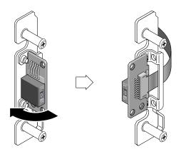
FIGURE 9-11 Removing the ID Switch Module
