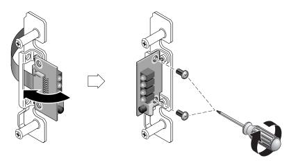
FIGURE 5-6 Installing the New LED Module
