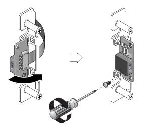
FIGURE 9-14 Installing the New ID Switch Module
