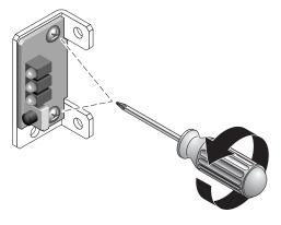
FIGURE 5-11 Removing the Screws Holding the LED Module
