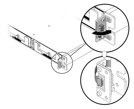
FIGURE 5-9 Removing the LED Module From the Chassis
