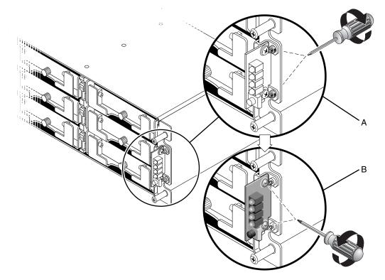
FIGURE 5-2 Detaching the LED Module From the Chassis
