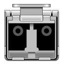
FIGURE 9-4 Duplex Jack at the End of an SFP
