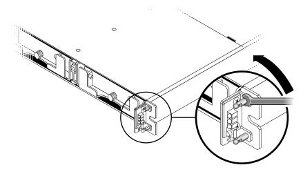
FIGURE 5-8 Removing the ball studs
