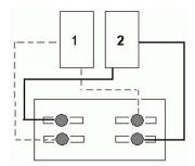
FIGURE 10-4 Example of a SCSI Array Configuration
