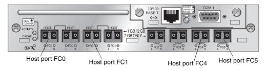
FIGURE 9-8 Sun StorEdge 3511 SATA Array Single-Controller SFP Placement
