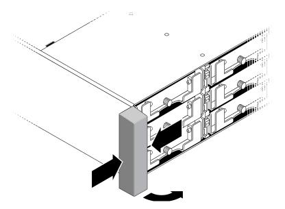
FIGURE 9-9 Removing the Left Ear Cap
