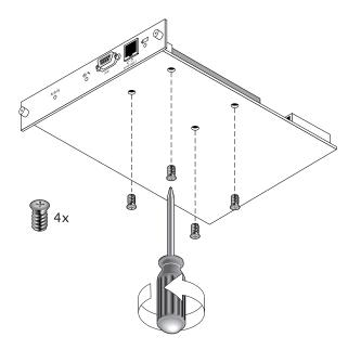
FIGURE 4-5 The Underside of the Battery Module With Screws Being Removed
