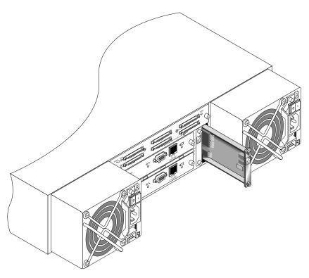
FIGURE 10-2 The EMU Module Partially Pulled out of the Chassis
