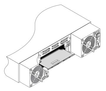
FIGURE 10-1 The Terminator Module Partially Pulled Out of the Chassis
