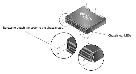
FIGURE 2-7 Attaching the Chassis Ears to the Tabletop Cover
