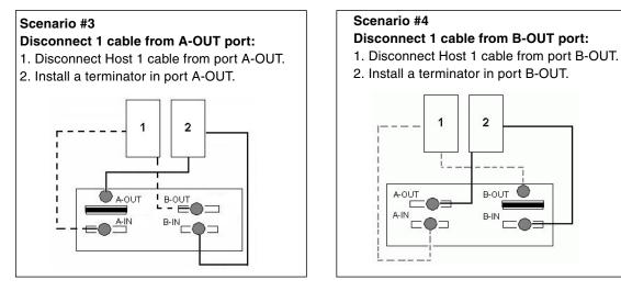
FIGURE 10-6 Removing a Single Cable From an OUT Port in a Two-Host Configuration
