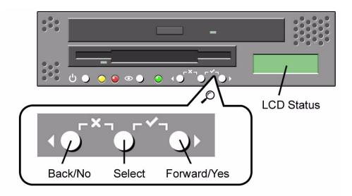
FIGURE 1-2 Operator Panel and Buttons
