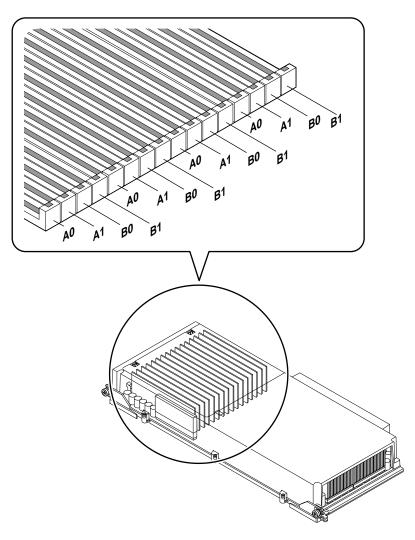
Qualified service technicians must physically remove a CPU/Memory board from the system before installing or removing DIMMs. The DIMMs must be added fourat-a-time within the same DIMM group and be identical—that is, all DIMMs must be from the same manufacturing vendor and must have the same capacity (for example, four 512-Mbyte DIMMs, or four 1-Gbyte DIMMs).
