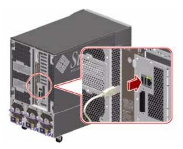
5. Attach the mouse cable to the system's remaining USB port, or to a USB port on the keyboard, if applicable.
