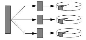
System performance using RAID 0 will be better than using RAID 1 or 5, but the possibility of data loss is greater because there is no way to retrieve or reconstruct data stored on a failed disk drive.
