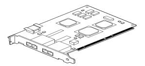
Sun StorEdge PCI Dual Fibre Channel Host Adapter Card
