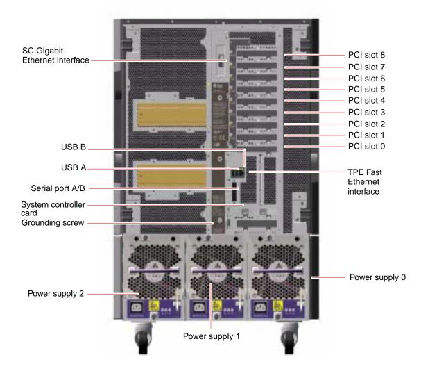
The three power supplies are accessible from the system rear panel. Each power supply has three LED indicators for displaying power status and fault conditions. See "About Power Supply LEDs" on page 145 for additional details.
