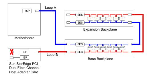
To provide additional hardware redundancy, two split backplane configurations are available as field-installed options. See the "Split Backplane Configurations" appendix in the *Sun Fire V890 Server Service Manual*.
