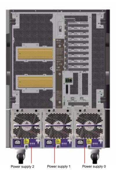
The system can accommodate a maximum of three power supplies, each with its own 10-amp AC power cord. Each power supply provides up to 1629 watts of DC power at 200-240 VAC line input. The basic system configuration comes with three power supplies installed. The third power supply provides N+1 power redundancy, allowing the system to continue operating should any one of the power supplies fail.
