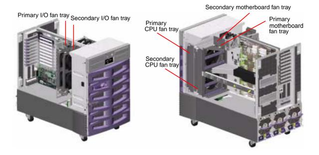
Only the primary fan trays are running during normal system operation. If a primary fan tray fails, the environmental monitoring subsystem detects the failure and automatically activates the secondary fan tray.
