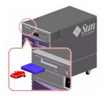
Do not use any cartridge other than a DDS-approved cleaning tape cartridge to clean your tape drive.
