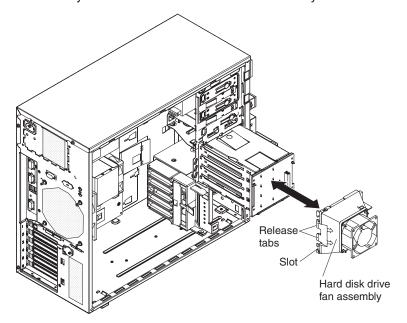
If you have the eight-drive, 2.5-inch hot-swap hard disk drive model, the hard disk drive fan assembly looks like the following illustration.
