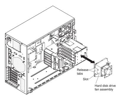
If you have the eight-drive, 2.5-inch hot-swap hard disk drive model, the hard disk drive fan assembly looks like the following illustration.
