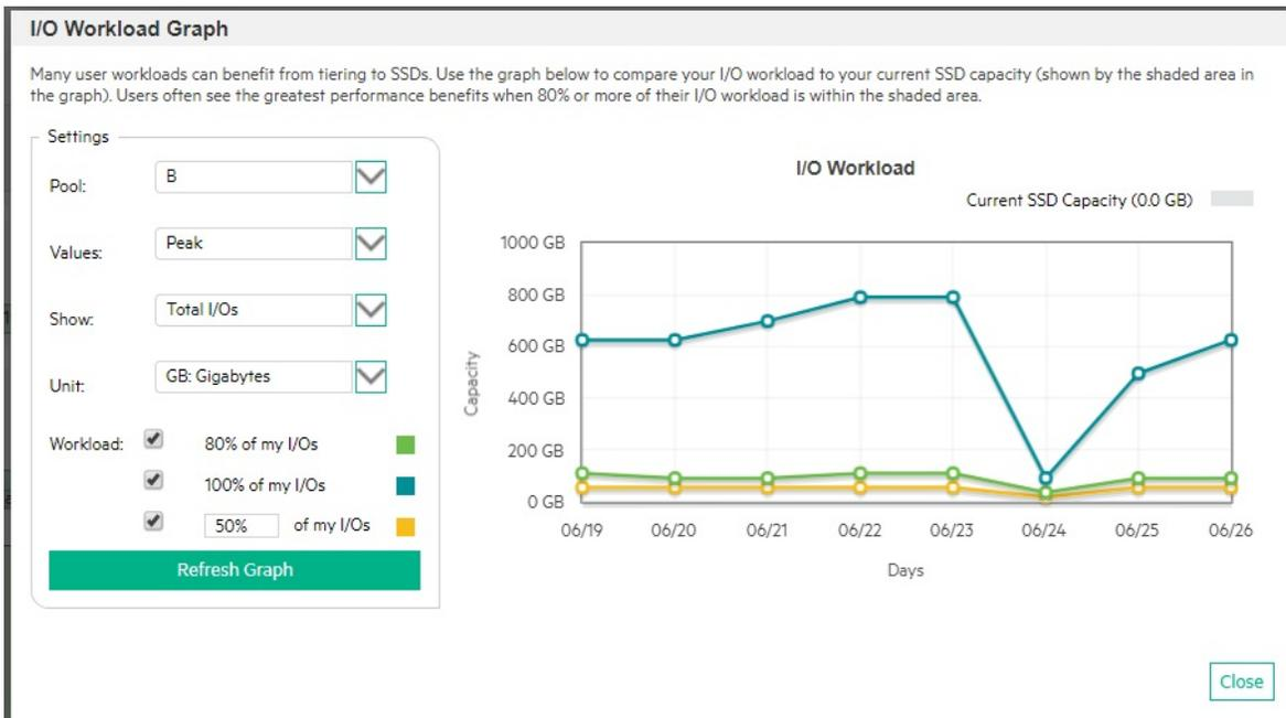
Figure 11. I/O Workload graph for Pool B
