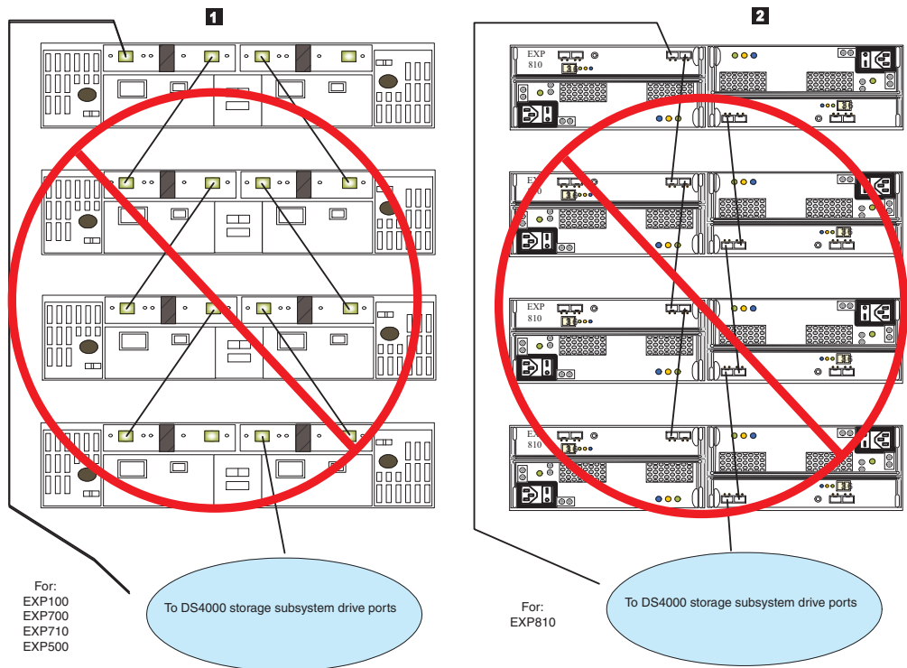
Figure 39. Unsupported cable loop scheme for connecting storage devices (1 of 2)
