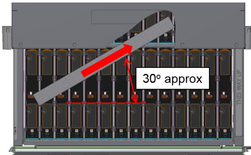
Figure 70. Keeping the strip contacting with the pop-up DDIC
