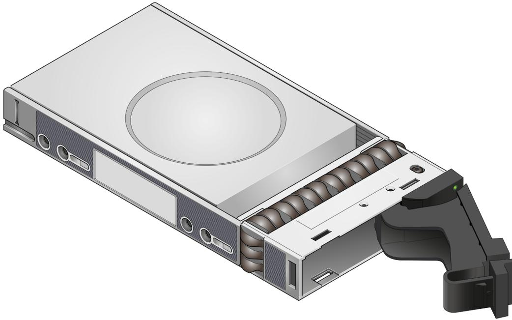
Figure 79. Installing a Drive Carrier Module (1)
