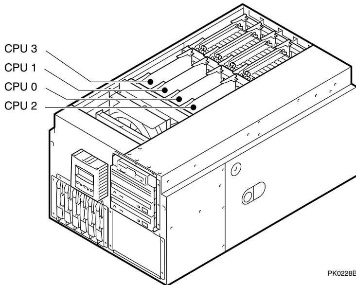
**Figure 4-8 CPU Slot Locations (Tower View)**
