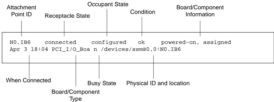
**FIGURE 9-1** Details of the Display for `cfgadm -av`
