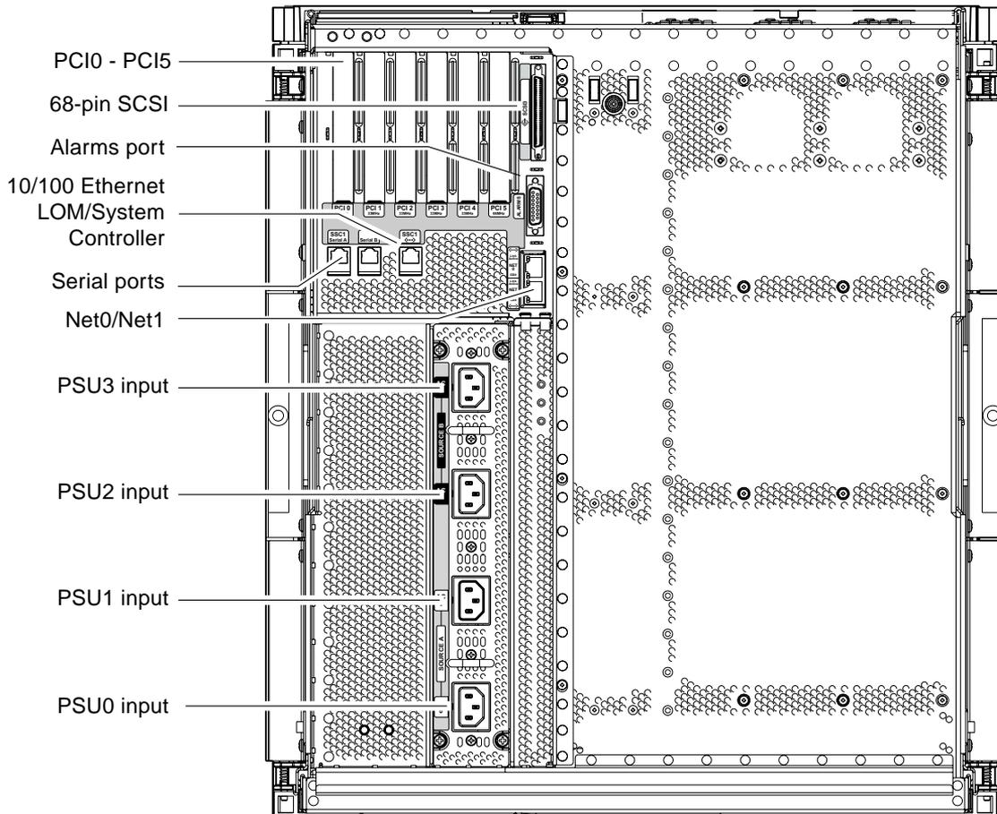
FIGURE 1-1 I/O Ports
