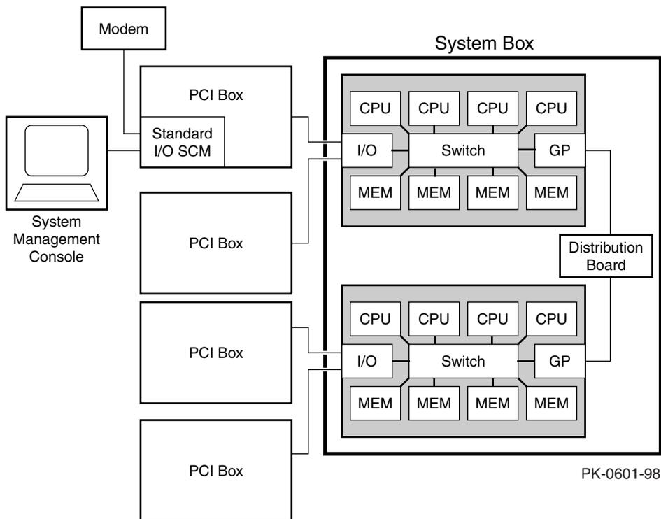
Figure 1–2 shows a block diagram of a GS160 with two system boxes. A hierarchical switch makes the interconnect between the QBBs in the two system boxes through their global ports.
