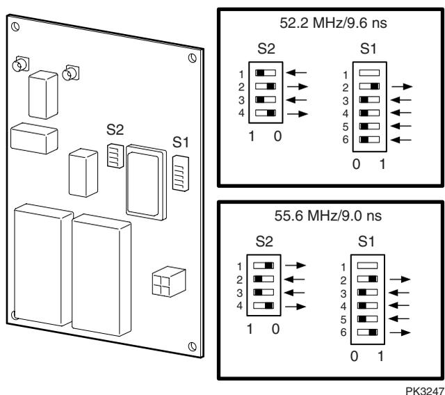
The switch packs on the master clock control the speed of the system. When B4125 CPUs are in the system, the clock runs at 9.6 ns. To set the system speed to 9.0 ns, access the clock module and change the switches.
