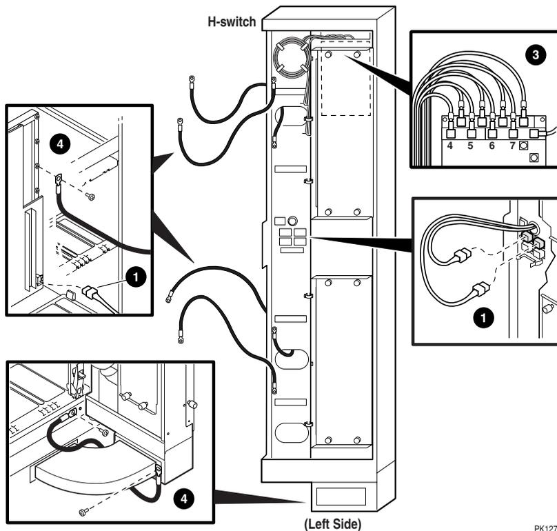
12. Remove and discard the filler plate from the right side of the H-switch bottom. Install plenum to the H-switch ❶ (Figure 3-8) using the filler plate mounting screw.
