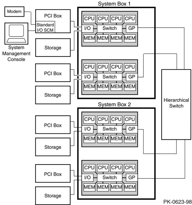
Figure 1-3 shows a block diagram of a GS320 with four system boxes. A hierarchical switch makes the interconnect between the QBBs in the four system boxes through their global ports.
