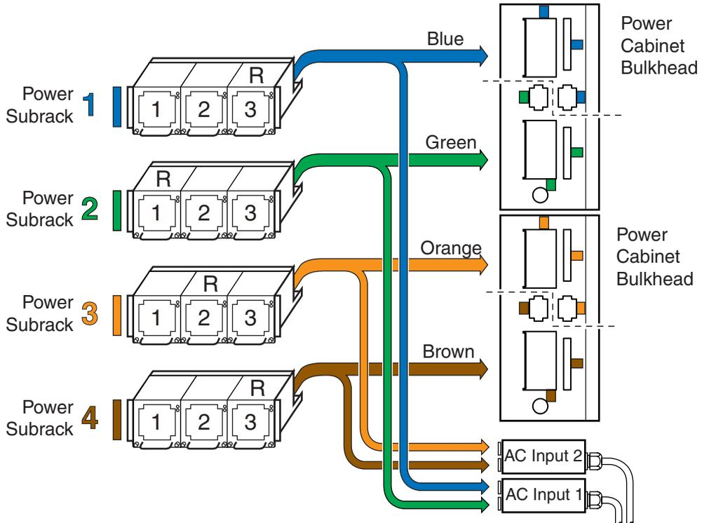
R indicates redundant power supply slot.
