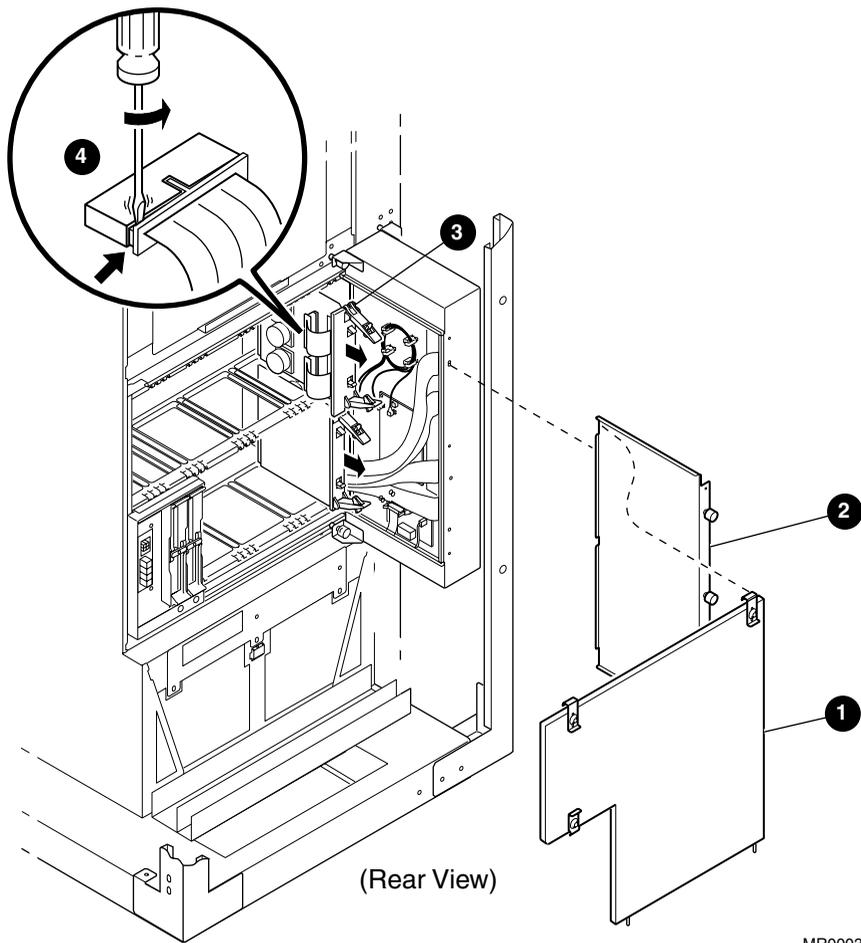
Remove the distribution board assembly as follows:
