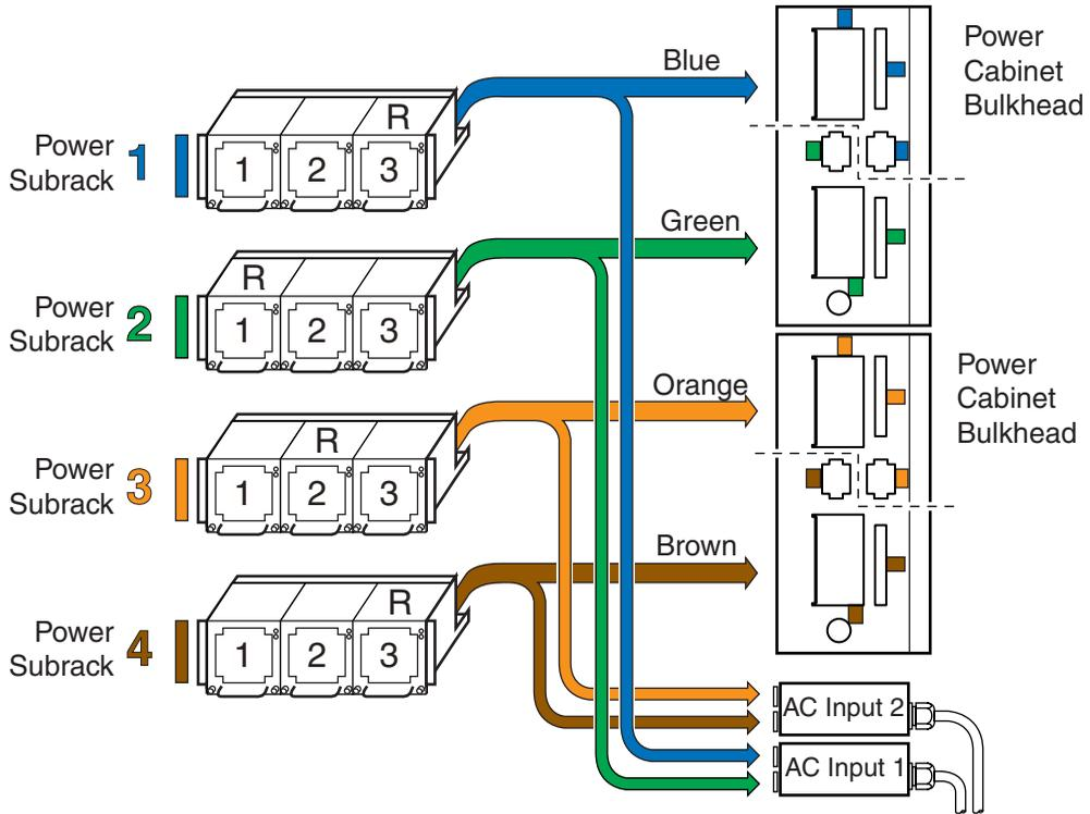
R indicates redundant power supply slot.
