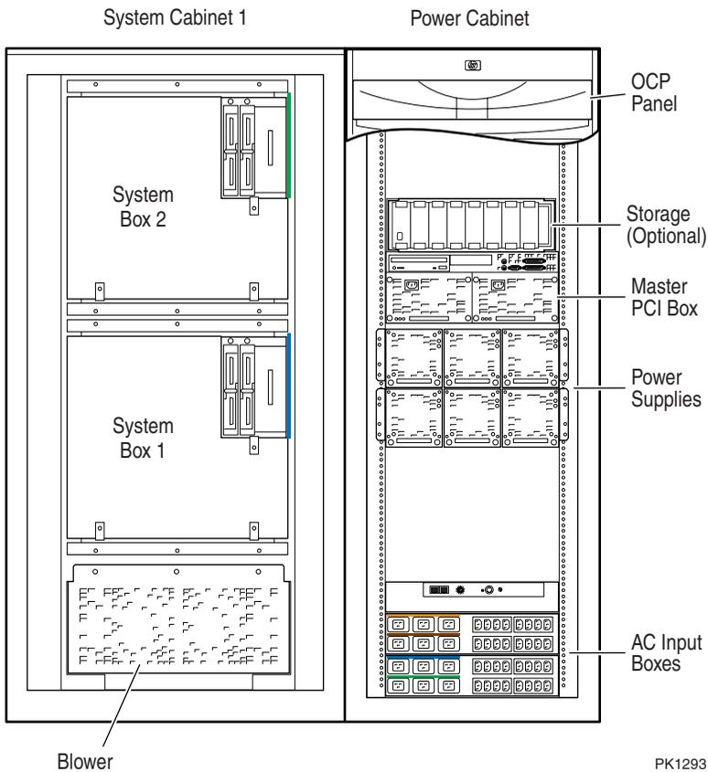
Figure 1-5 shows a fully configured GS320 system.
