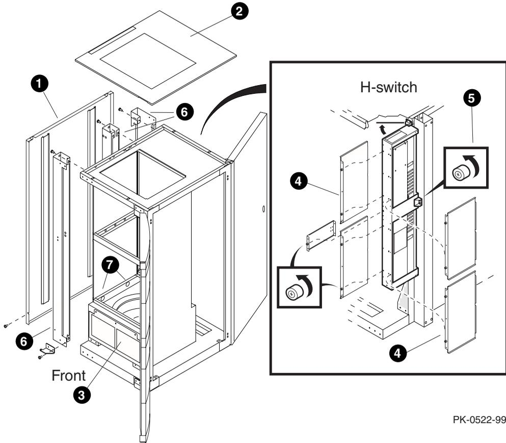
Position system cabinet 1 at the predetermined location. Lower the corner leveling feet on system cabinet 1 until the system cabinet is anchored and the casters are free to rotate. Release the tie wraps on the CSB cable and hose cables that are coiled and attached to the sides of system cabinets for later routing.
