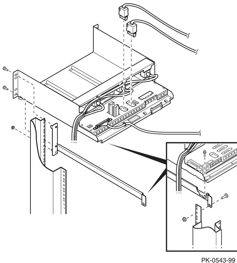
Install the power subrack into the cabinet as follows:
