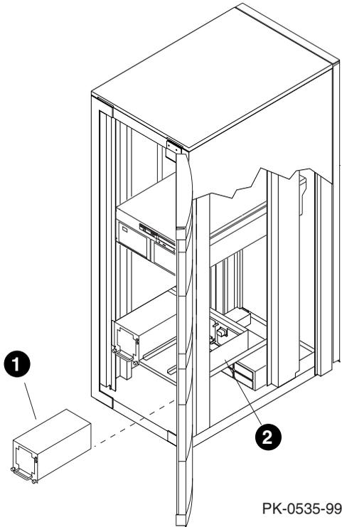
Each power subrack requires a minimum of two power supplies. A redundant third power supply is recommended. Figure 5–17 shows the power supply slot assignments and the placement of the three power supplies for each of the four power subracks.
