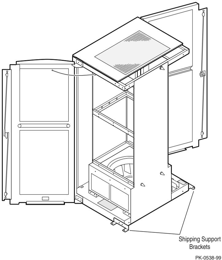
System cabinet 2 is similar to system cabinet 1. It contains up to two system boxes. It is joined to system cabinet 1 to expand the system configuration from two system boxes to three or four system boxes.
