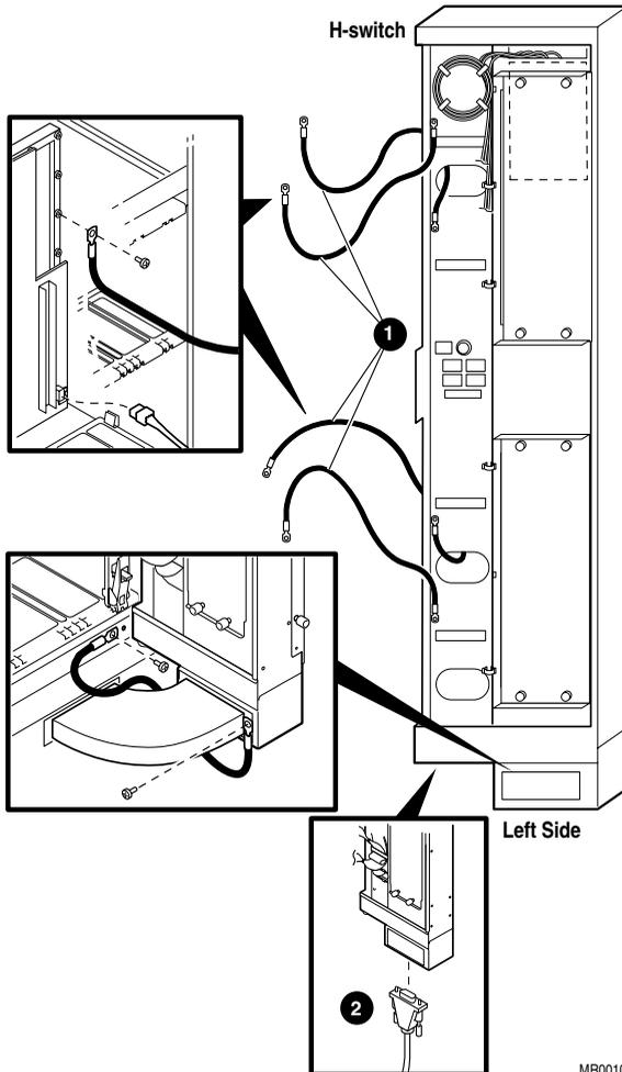
Attach the ground cables and the CSB cable as shown in Figure 2–7:
