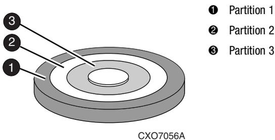
Figure 2-17. One example of a partitioned single-disk unit
