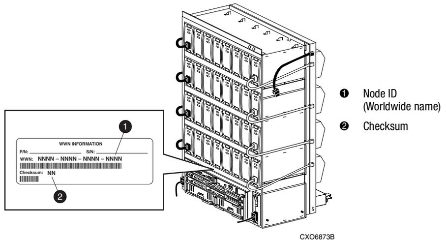
Figure 1-16. Placement of the worldwide name label on the BA370 enclosure
