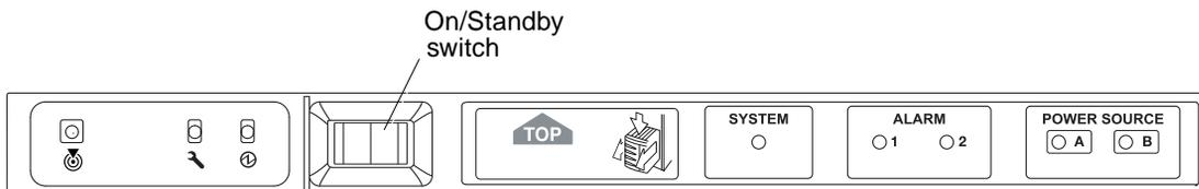
**FIGURE 2-1** Netra 1290 Server On/Standby Switch
