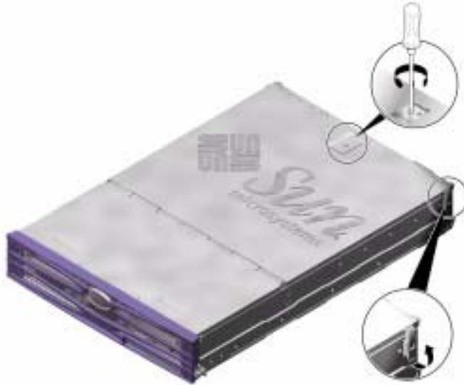
FIGURE 2-2 Lifting the lid
