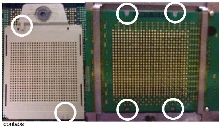
2. Guide pins are provided on the processor extender board to assist in alignment. While these pins do not assure precise alignment, they will position the CPU module for installation. Check that the guide pins intact and free of debris before starting. Check that the corresponding holes in the CPU module are clean and free of debris before starting.
