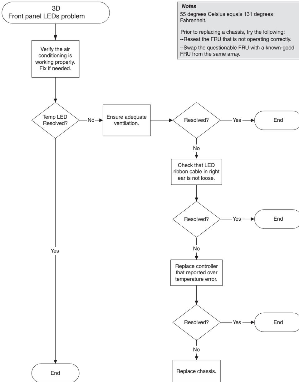
FIGURE 8-9 Front Panel LEDs Flowchart, 4 of 4
