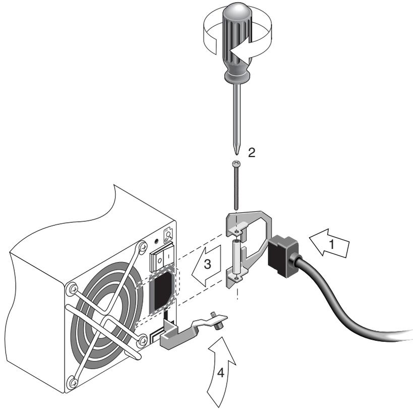
**FIGURE 4-5** Connecting the Chassis to AC Power
