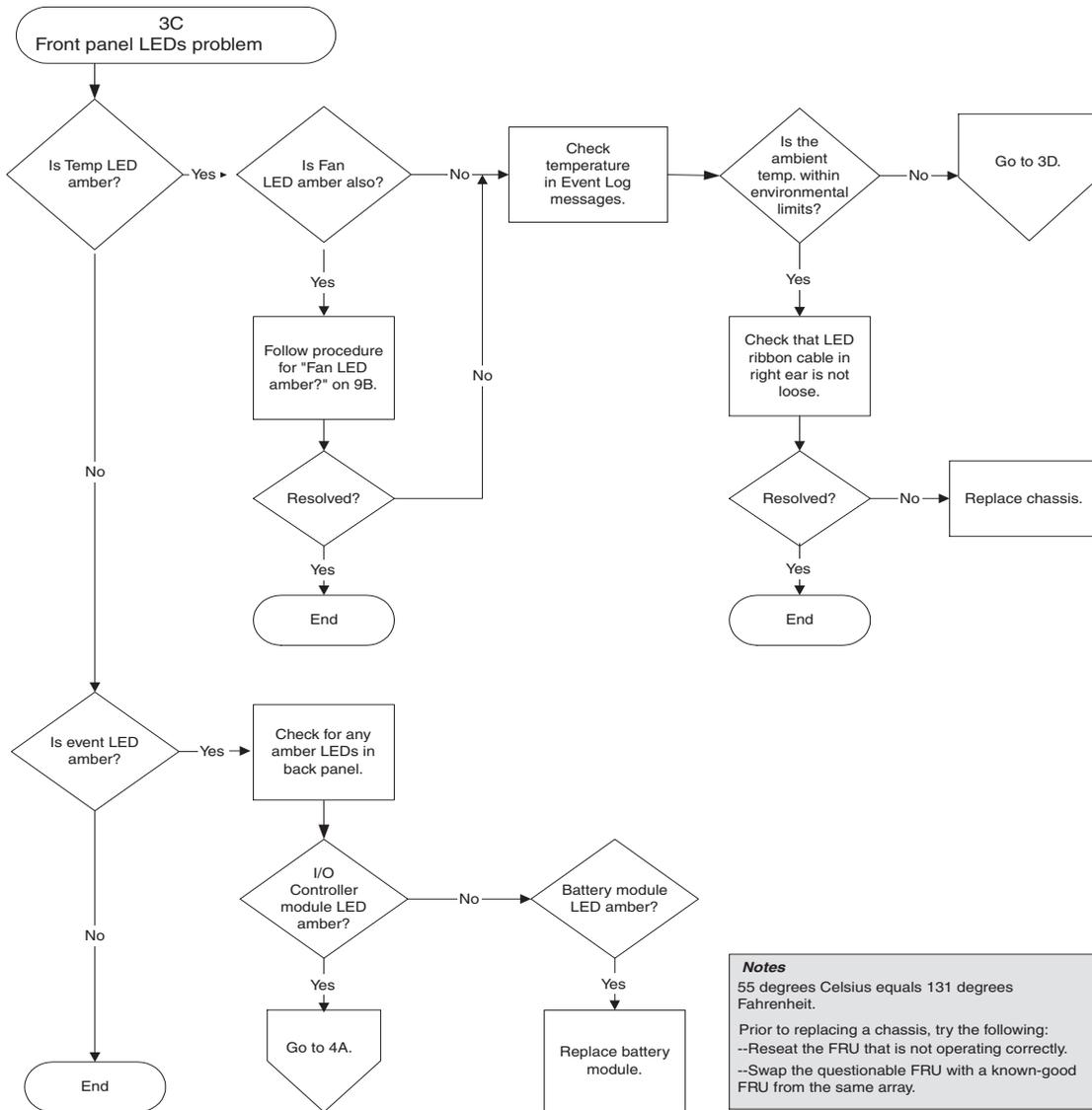
**FIGURE 8-8** Front Panel LEDs Flowchart, 3 of 4
