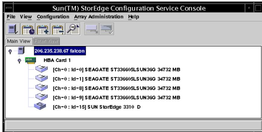
In a split-bus configuration, each port is connected to its own HBA, as shown in the following example:
