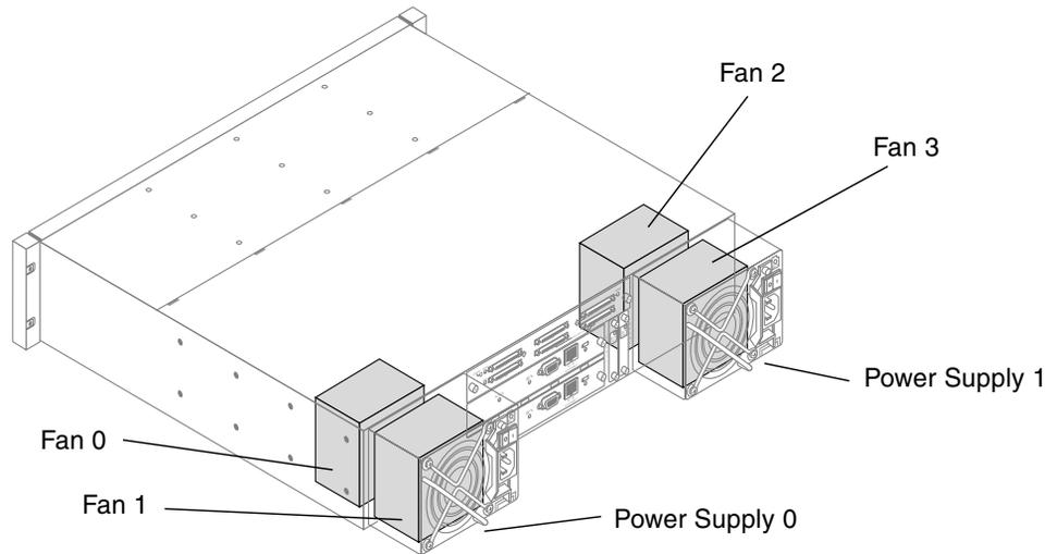
**FIGURE 8-1** Cooling Fan and Power Supply Locations
