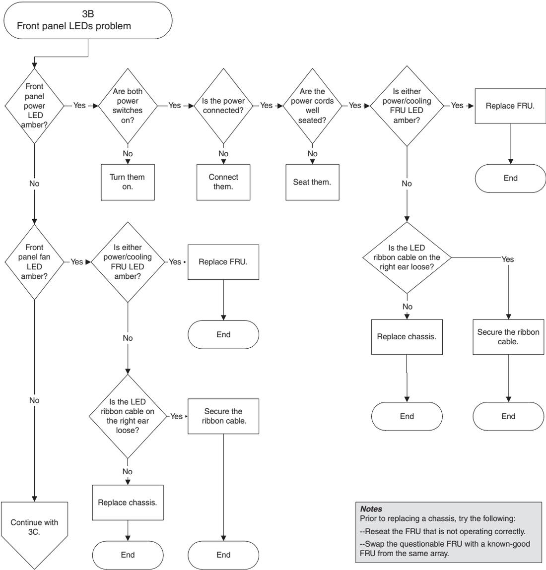
**FIGURE 8-7** Front Panel LEDs Flowchart, 2 of 4
