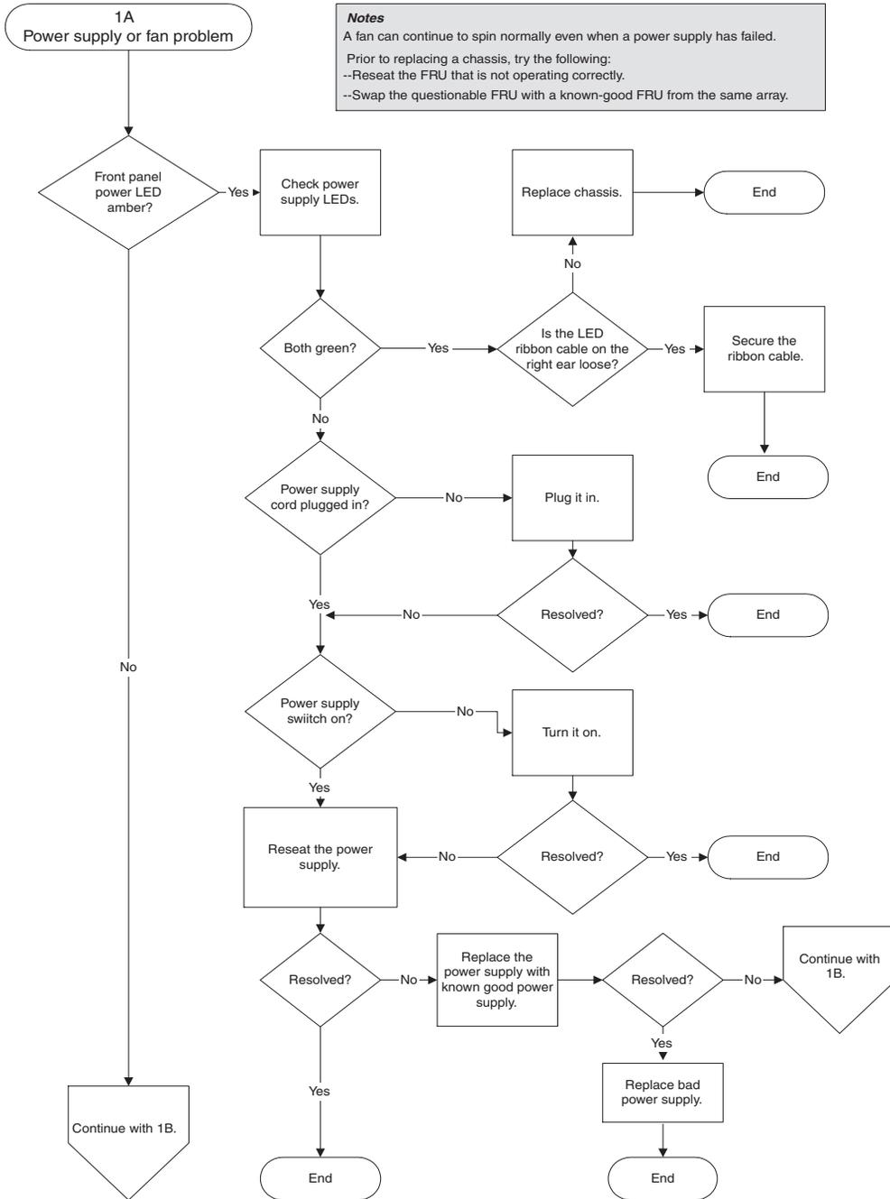
**FIGURE 8-2** Power Supply or Fan Module Flowchart, 1 of 2
