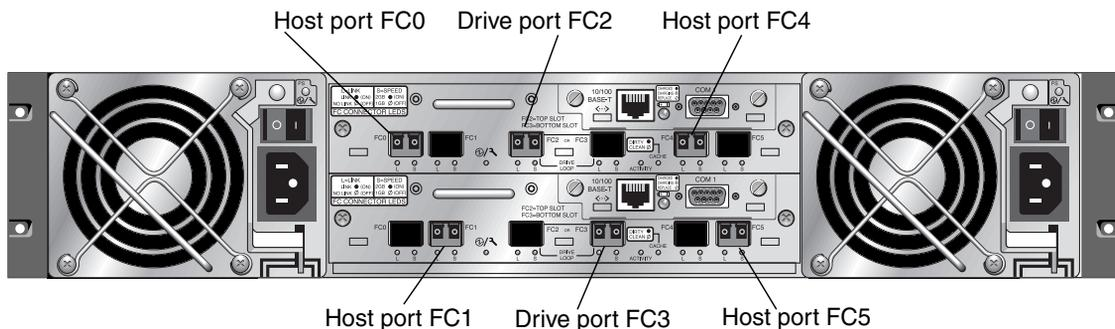
**FIGURE 4-15** Default Dual-Controller Sun StorEdge 3510 FC Array SFP Placement
