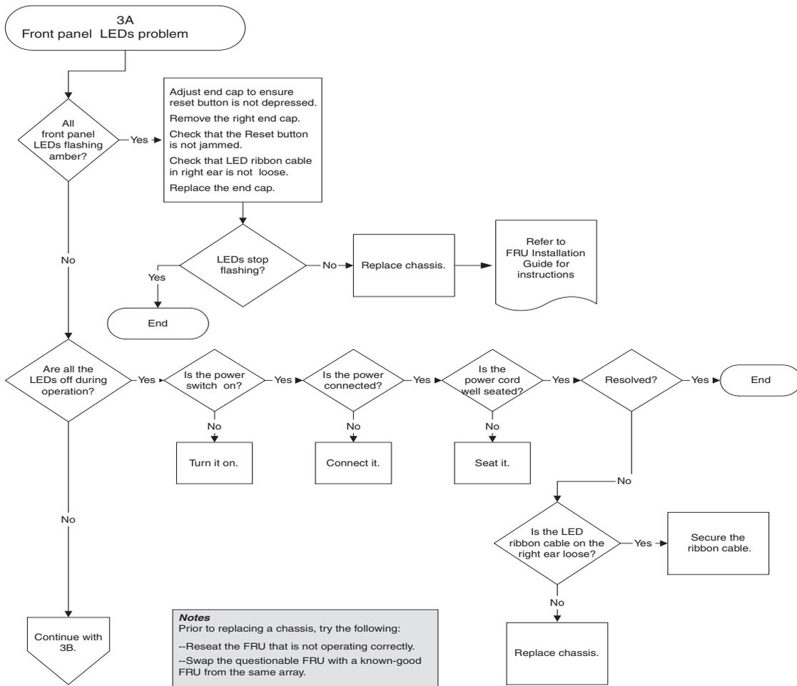
**FIGURE 8-6** Front Panel LEDs Flowchart, 1 of 4
