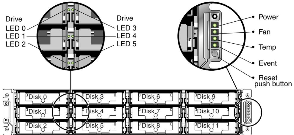
**FIGURE 6-1** Front Panel LEDs
