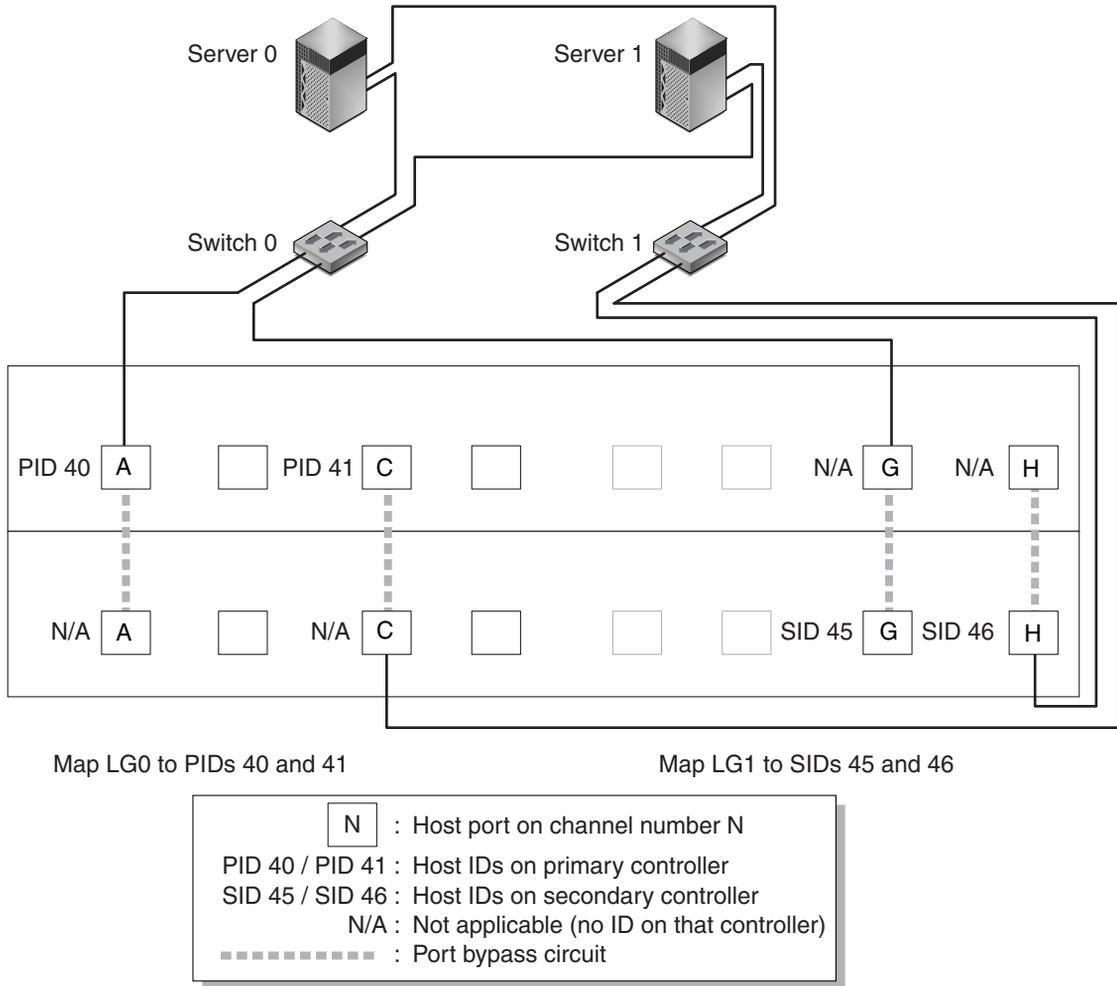
**FIGURE 5-2** A Point-to-Point Configuration With a Dual-Controller Sun StorEdge 3511 SATA Array and Two Switches
