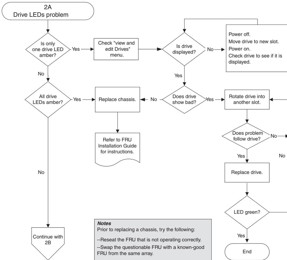
FIGURE 8-4 Drive LEDs Flowchart, 1 of 2
