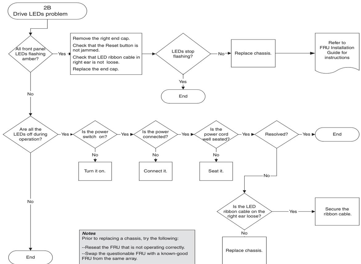
FIGURE 8-5 Drive LEDs Flowchart, 2 of 2
