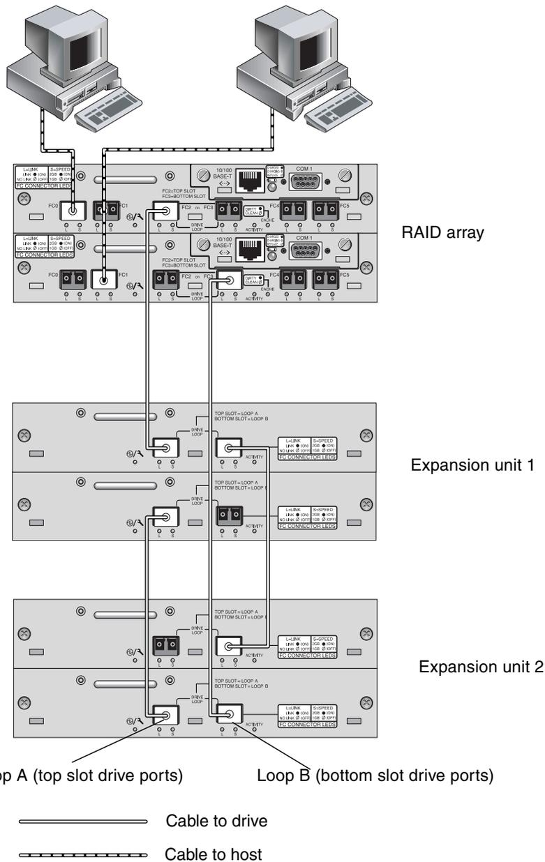
**FIGURE 4-6** Sun StorEdge 3510 FC Array Attached to Two Hosts and Two Expansion Units
