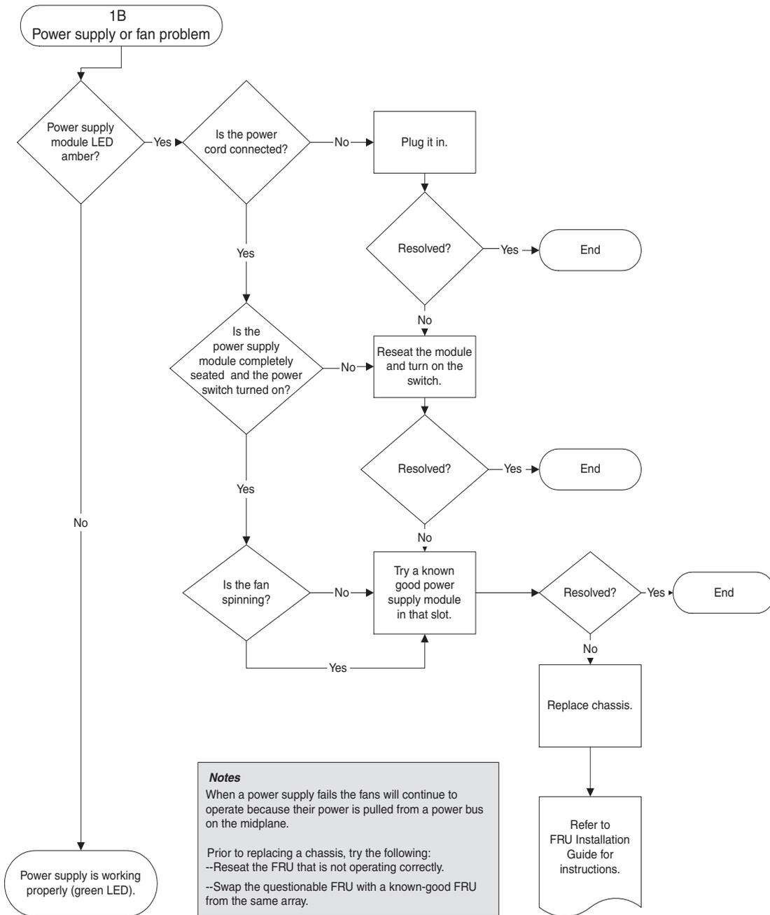
FIGURE 8-3 Power Supply or Fan Module Flowchart, 2 of 2
