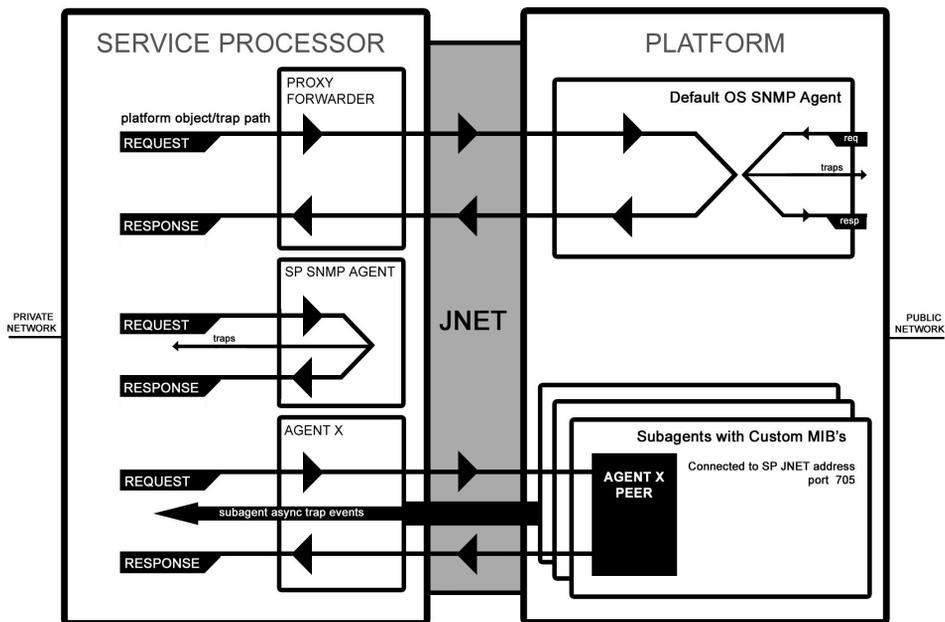
**FIGURE 3-2** SNMP Architecture and Communications
