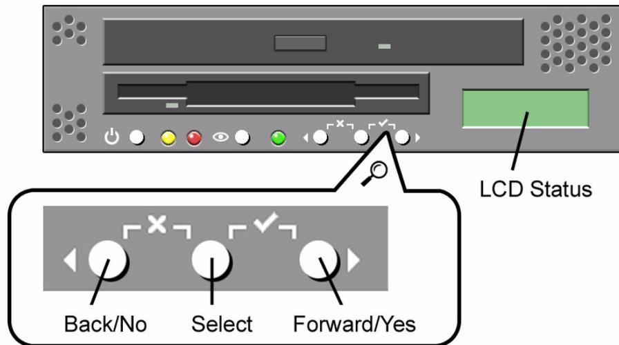
FIGURE 1-2 Operator Panel and Buttons
