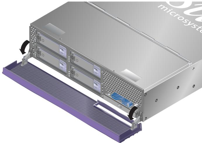
**FIGURE 2-2** Opening The Bezel (Sun Fire V240 Server)
