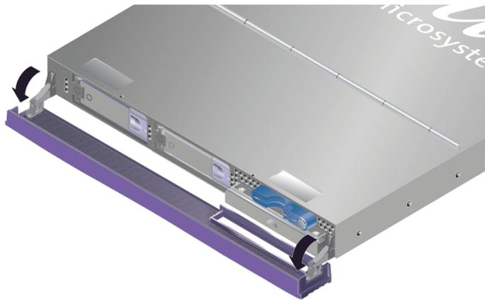
**FIGURE 2-1** Opening the Bezel (Sun Fire V210 Server)
