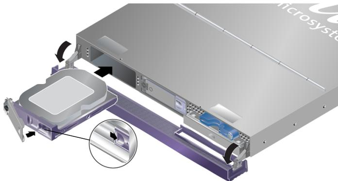
**FIGURE 2-4** Installing a Hard Drive (Sun Fire V210 Server)
