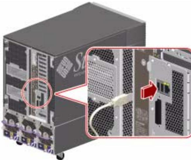
5. **Attach the mouse cable to the system's remaining USB port, or to a USB port on the keyboard, if applicable.**
