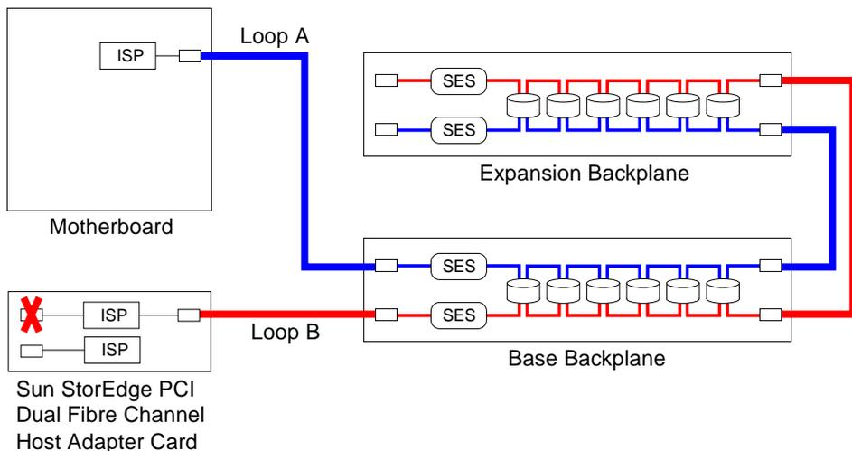
To provide additional hardware redundancy, two split backplane configurations are available as field-installed options. See the “Split Backplane Configurations” appendix in the *Sun Fire V890 Server Service Manual*.
