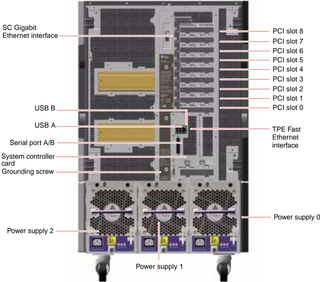
The three power supplies are accessible from the system rear panel. Each power supply has three LED indicators for displaying power status and fault conditions. See “About Power Supply LEDs” on page 145 for additional details.
