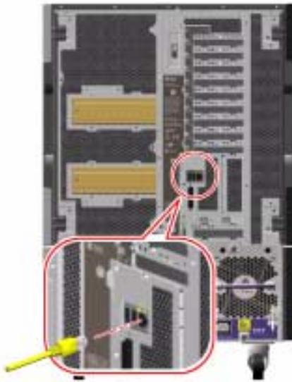
**3. Connect the other end of the cable to the RJ-45 outlet to the appropriate network device.**
