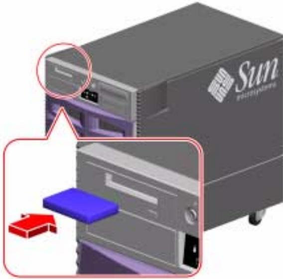
Do not use any cartridge other than a DDS-approved cleaning tape cartridge to clean your tape drive.
