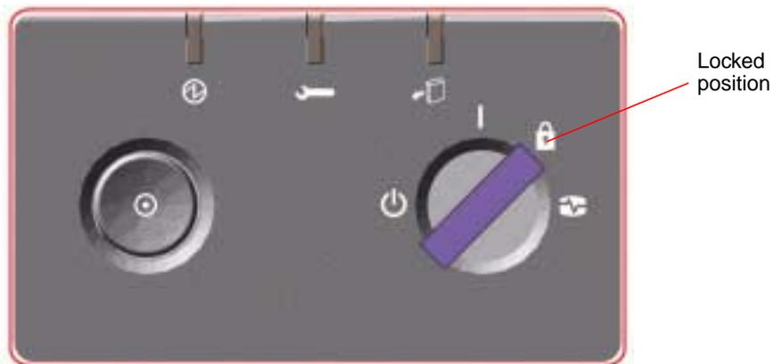
6. Remove the key from the keyswitch and keep it in a secure place.
