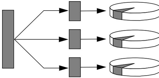
System performance using RAID 0 will be better than using RAID 1 or 5, but the possibility of data loss is greater because there is no way to retrieve or reconstruct data stored on a failed disk drive.
