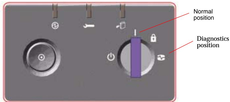
4. **Press and release the Power button on the system front panel.**
