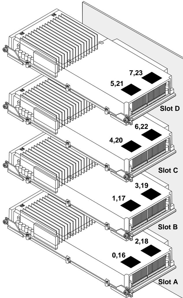
The UltraSPARC IV processor is a high-performance, highly integrated, CMP processor that enables an increase in application throughput while maintaining binary compatibility. The UltraSPARC IV processor implements a 64-bit SPARC International Version 9 Instruction Set Architecture (ISA).
