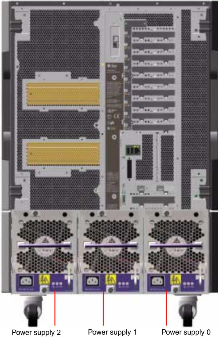
The system can accommodate a maximum of three power supplies, each with its own 10-amp AC power cord. Each power supply provides up to 1629 watts of DC power at 200-240 VAC line input. The basic system configuration comes with three power supplies installed. The third power supply provides N+1 power redundancy, allowing the system to continue operating should any one of the power supplies fail.
