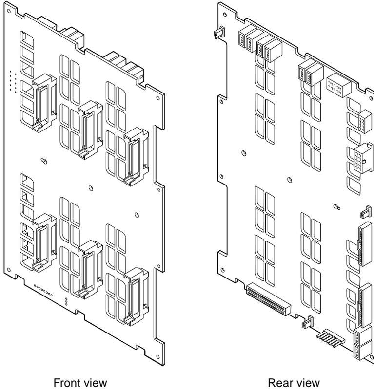
The FC-AL backplane accepts low-profile (1.0-inch) dual-ported FC-AL disk drives. Each disk drive connects to the backplane via a standard 40-pin single connector attachment (SCA) interface. Incorporating all power and signal connections into a single, blind-mating connector, SCA technology makes it easy to add or remove disk drives from the system. Disks using SCA connectors provide higher availability and better serviceability than disks using other types of connectors.
