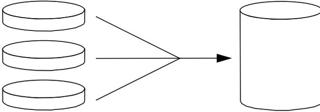
Using this method, the concatenated disks are filled with data sequentially, with the second disk being written to when no space remains on the first, the third when no room remains on the second, and so on.
