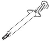
**Note:** If the grease is properly applied, approximately half of the grease will remain in the syringe.
