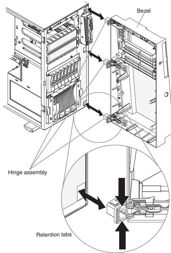
**Note:** The bezel also disengages from the chassis hinges if you rotate the bezel beyond 180° or if excessive pressure is applied to the bezel. Do not be alarmed, because this is how the bezel was designed. The bezel is designed with breakaway hinges so that you can easily reattach it to the chassis.
