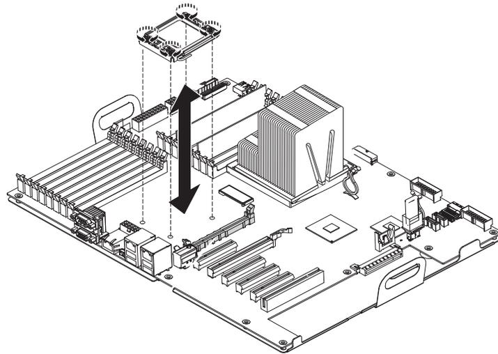
To remove a microprocessor retention module, complete the following steps:
