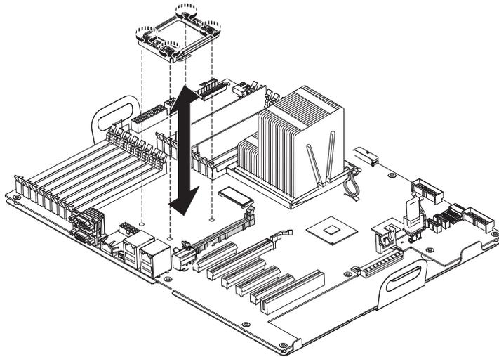
To install a microprocessor retention module, complete the following steps:
