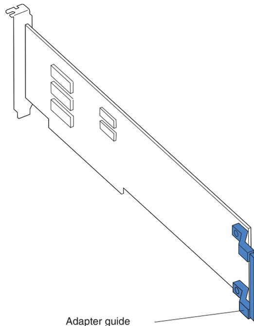
6. Press the adapter *firmly* into the expansion slot.
