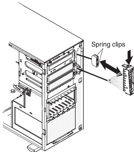
To remove the USB cable and light path diagnostics assembly from the server, complete the following steps:
