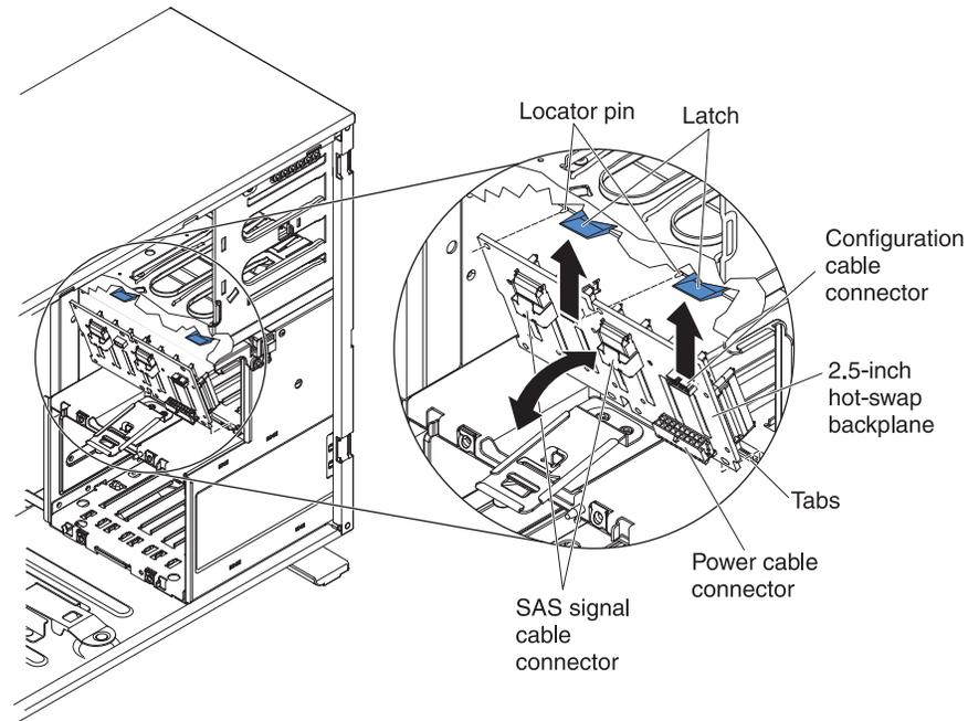
3. Connect the power, signal, and configuration cables to the 2.5-inch hard disk drive backplane (see “Hard disk drive backplane connectors” on page 20 and “Internal cable routing and connectors” on page 169).
