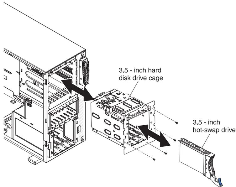
8. Align the holes in the edge of 3.5-inch disk drive cage with the holes in the edge of the server rack.
