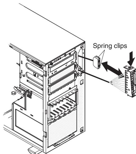
To install the USB cable and light path diagnostics assembly, complete the following steps:
