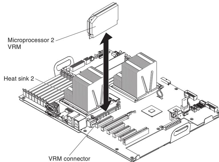
To install a voltage regulator module, complete the following steps:
