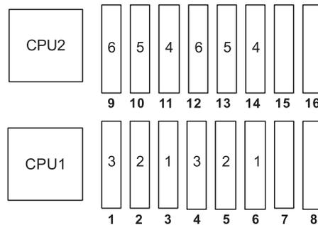
The following table lists the installation sequence for installing DIMMs in memory-mirroring mode.
