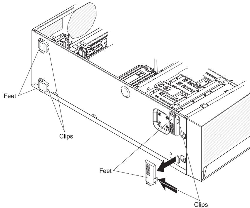
To rotate the front feet, complete the following steps:
