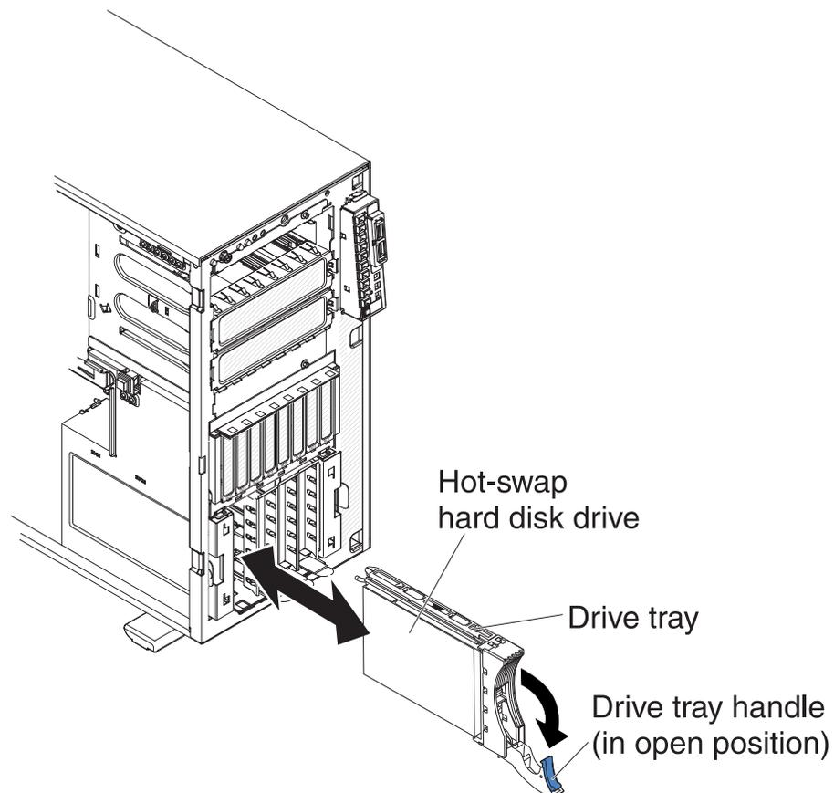
5. Rotate the drive tray handle to the closed position.
