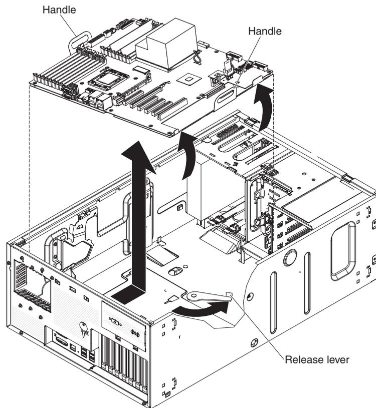
To remove the system board, complete the following steps:
