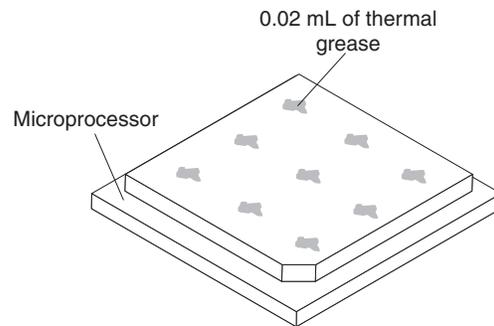
5. Use the thermal-grease syringe to place 9 uniformly spaced dots of 0.02 mL each on the top of the microprocessor. The outermost dots must be within approximately 5 mm of the edge. This is to ensure uniform distribution.
