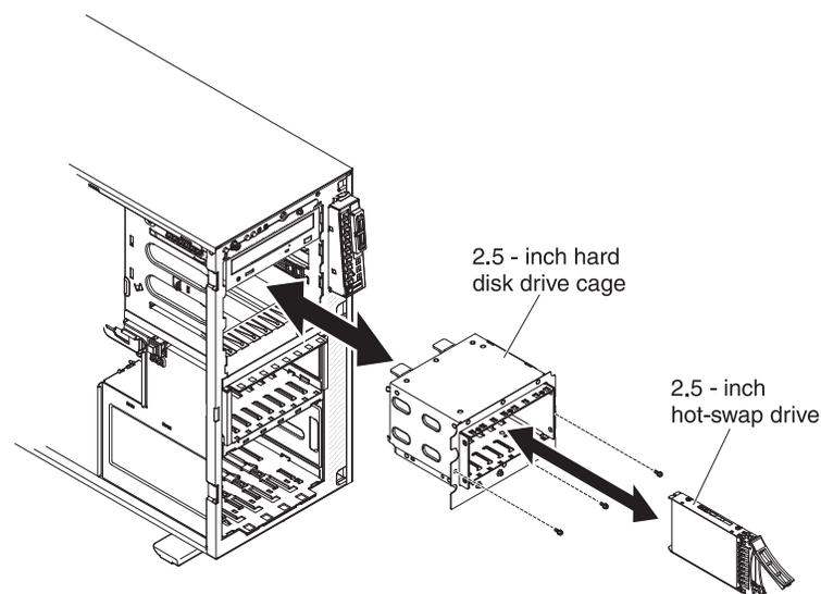
7. Insert the screws to secure the 2.5-inch disk drive cage in place.
