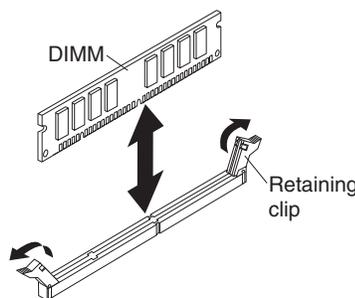
To remove a dual inline memory module (DIMM), complete the following steps:
