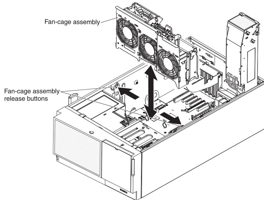
To remove the fan cage assembly, complete the following steps:
