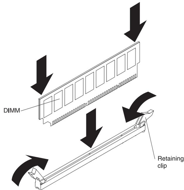
6. Firmly press the DIMM straight down into the connector by applying pressure on both ends of the DIMM simultaneously. The retaining clips snap into the locked position when the DIMM is firmly seated in the connector.
