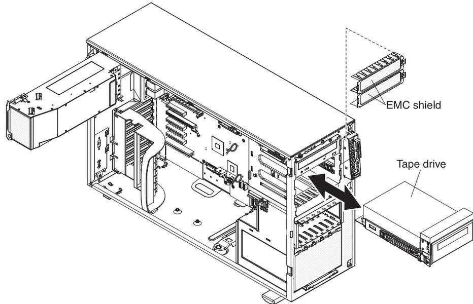
To install an optional full-height tape drive, complete the following steps:
