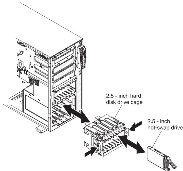
4. Install any hot-swap hard disk drives that were removed from the drive cage (see “Installing a 2.5-inch hot-swap hard disk drive” on page 196).
