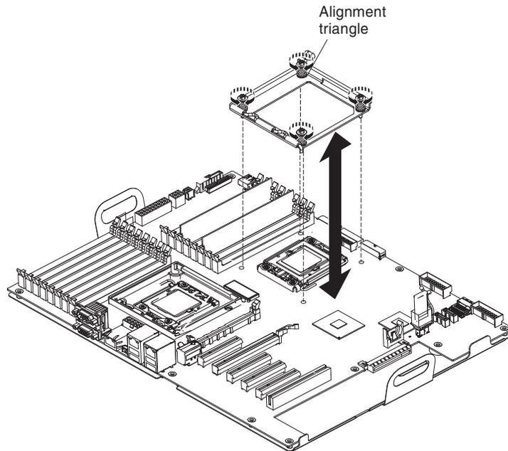
To install a heat-sink retention module, complete the following steps:
