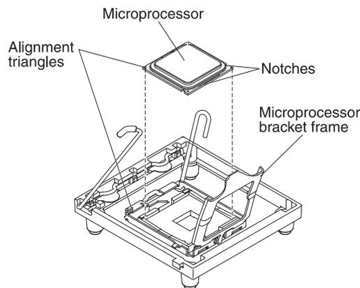
3. Open the microprocessor bracket frame and remove the microprocessor filler, if one is installed.
