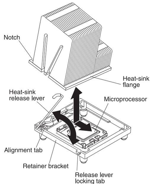
9. Lift the microprocessor-release latch to the fully open position (approximately 135° angle); then, lift the bracket frame and remove the microprocessor from the socket.
