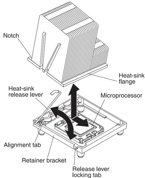
**Attention:** The heat sink is keyed to the retention module. Make sure that the notch on the heat sink fits over the alignment tab on the retention module.
