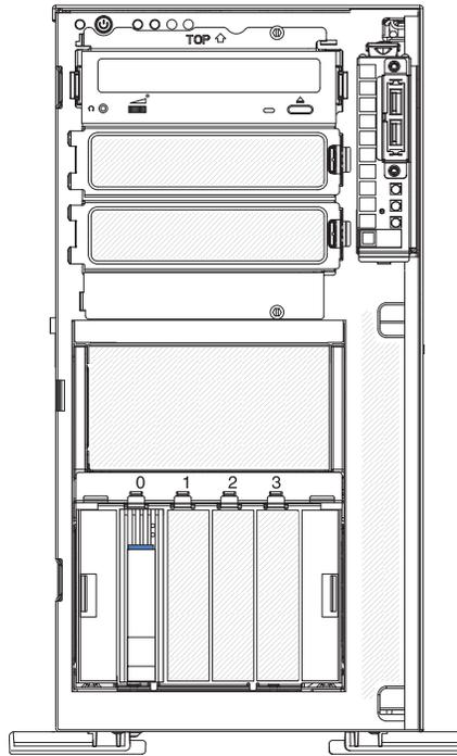
Figure 11. server with four 3.5-inch hard disk drives
