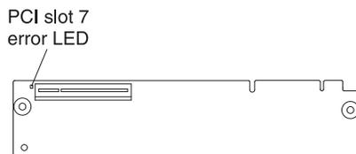
The following illustration shows the LEDs on the PCI-X extender card, if equipped.
