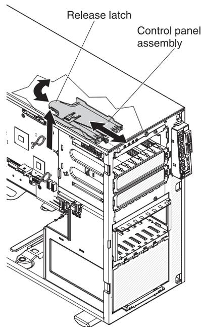
To install the operator information panel assembly, complete the following steps:
