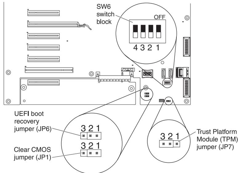
**Attention:** Before you change any switch settings or moving any jumpers, turn off the server; then, disconnect all power cords and external cables. See the safety information that begins on page “Safety” on page vii. Do not change settings or move jumpers on any system board switch or jumper blocks that are not shown in this document.
