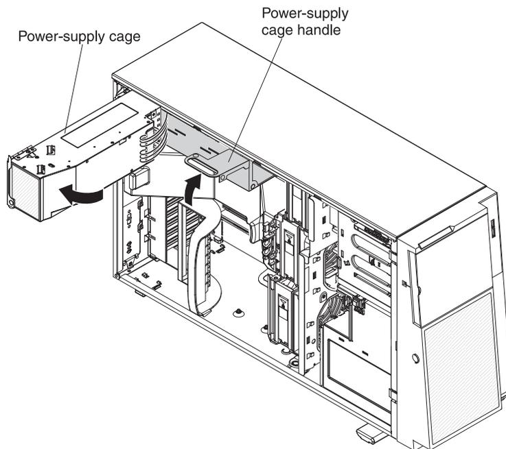
Opening the power-supply cage allows access to the air baffle, microprocessors, and DIMMs. To open the power-supply cage, complete the following steps:
