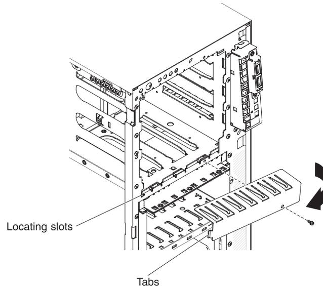
3. Touch the static-protective package that contains the 2.5-inch disk drive cage to any unpainted metal surface on the server; then, remove the drive cage from the package.
