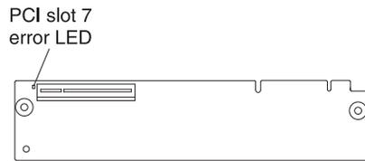
The following illustration shows the LEDs on the PCI-X extender card, if one is installed.
