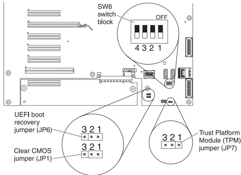
5. Remove any adapters that impede access to the UEFI boot recovery jumper block (JP6) (see “Removing an adapter” on page 219).
