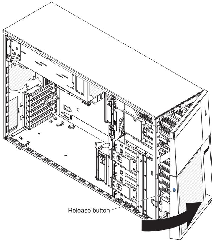
4. Press the retention tabs on each hinge assembly toward each other and pull the hinge assemblies out of the chassis.
