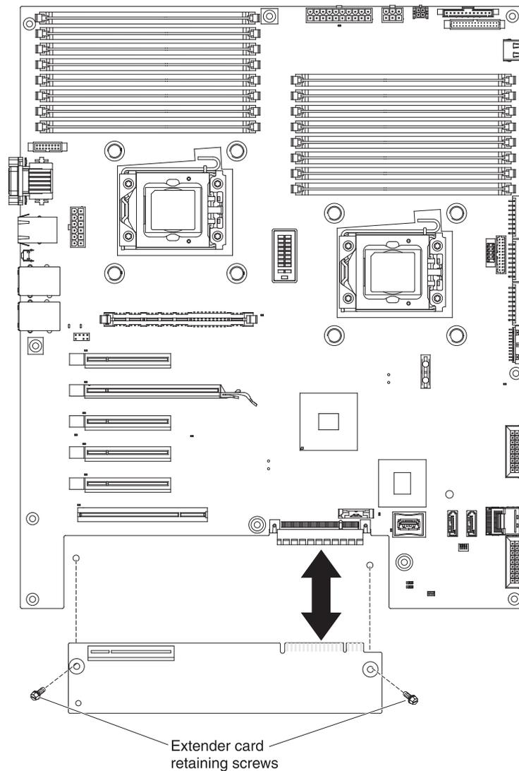
To remove an extender card, complete the following steps:
