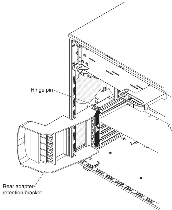
To remove the rear adapter-retention bracket, complete the following steps:
