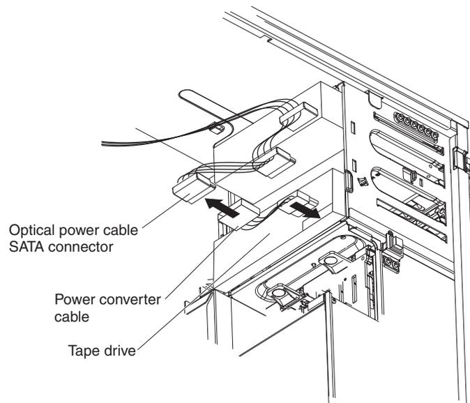
6. Connect one end of the tape drive signal cable to the tape drive and the other end to the connector on the system board. Route the cable through the plastic slots on the bottom of the chassis underneath the fan cage assembly. For more information, see *Internal cable routing and connectors*.
