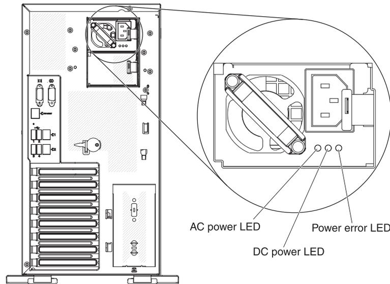
The following table describes the problems that are indicated by various combinations of the power-supply LEDs and the system power LED on the operator information panel and suggested actions to correct the detected problems.
