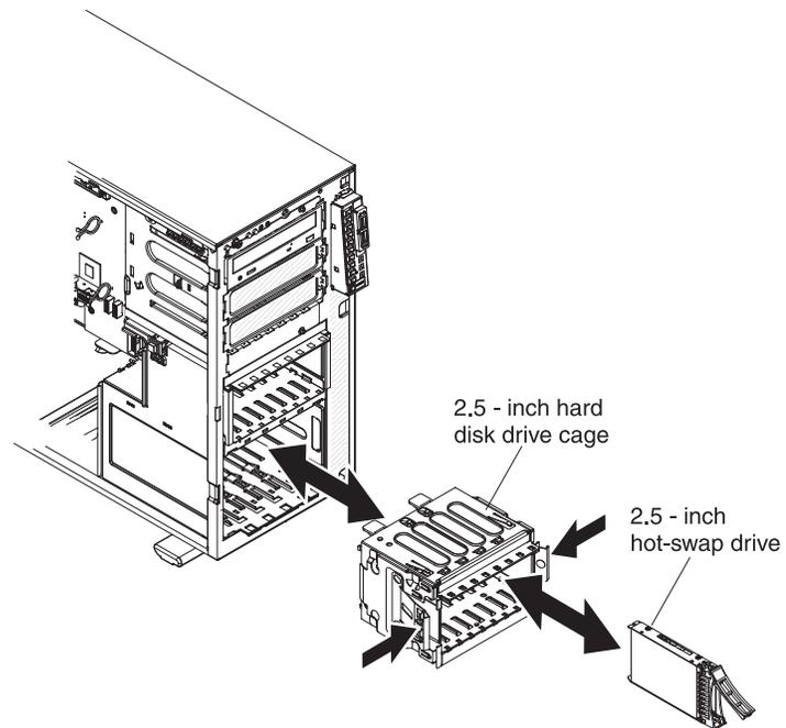
13. Remove the backplane from the 2.5-inch disk drive cage (see “Removing a 2.5-inch disk drive backplane” on page 257).
