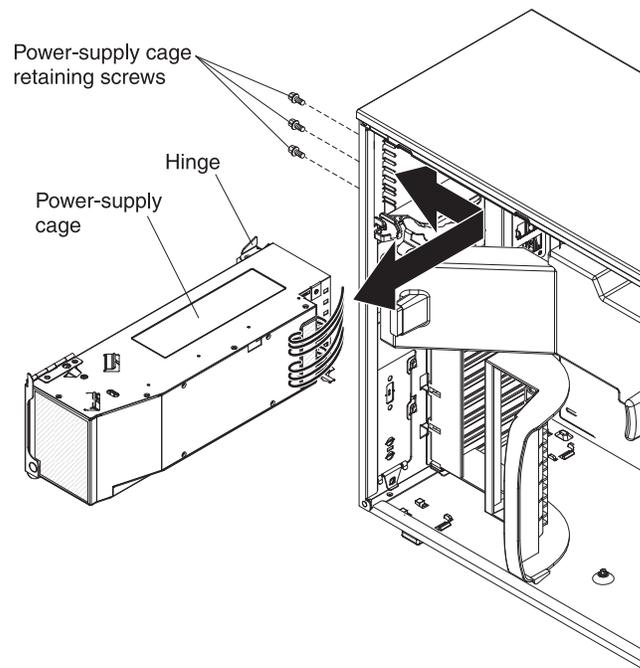
To install the power-supply cage, complete the following steps:
