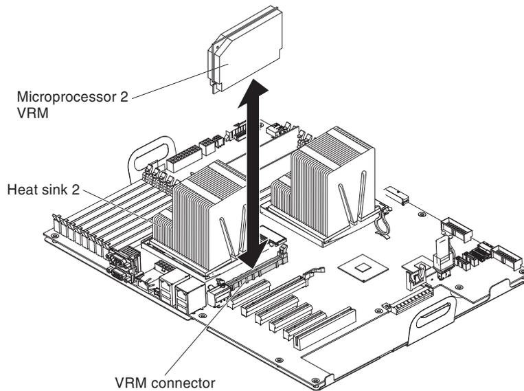
To remove a voltage regulator module (VRM), complete the following steps:
