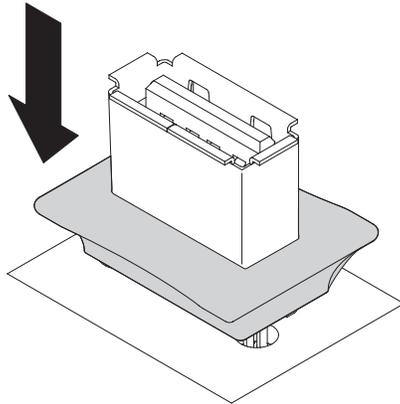
5. Align the flash device with the USB connector on the system board and push it into the USB connector until it is firmly seated.
