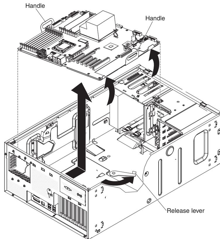
To install the system board, complete the following steps:
