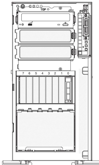
Figure 8. server with eight 2.5-inch hard disk drives
