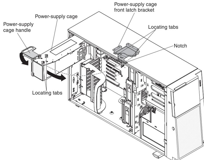
3. Rotate the power-supply cage handle down until the handle tip engages the notch in the front latch bracket; then, lower the handle until it locks in place.
