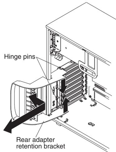
To install the rear adapter-retention bracket, complete the following steps:
