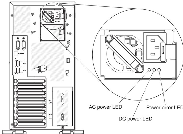
The following table describes the problems that are indicated by various combinations of the power-supply LEDs. For more information about solving power-supply problems, see “Power-supply LEDs” on page 99.
