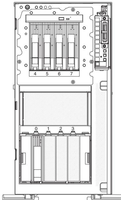
Figure 12. server with eight 3.5-inch hard disk drives
