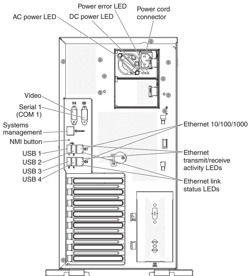
**AC power LED:** This green LED provides status information about the power supply. During typical operation, both the AC and DC power LEDs are lit.
