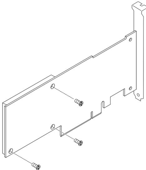
8. Install the ServerRAID adapter on the system board (see “Installing an adapter” on page 220).
