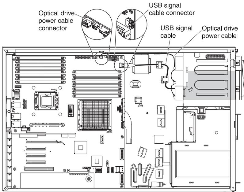
The following illustrations show the cabling information for installing the SATA to traditional power converter cable when you install an RDX internal USB tape drive in the server. This cable comes with the server in the plastic bag with the drive rails.
