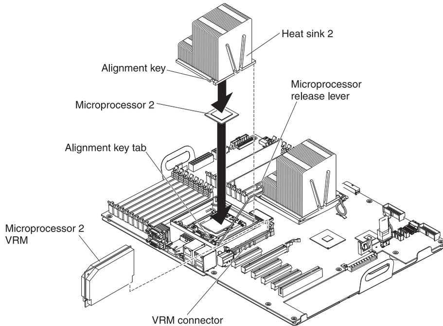
To install a microprocessor, complete the following steps:
