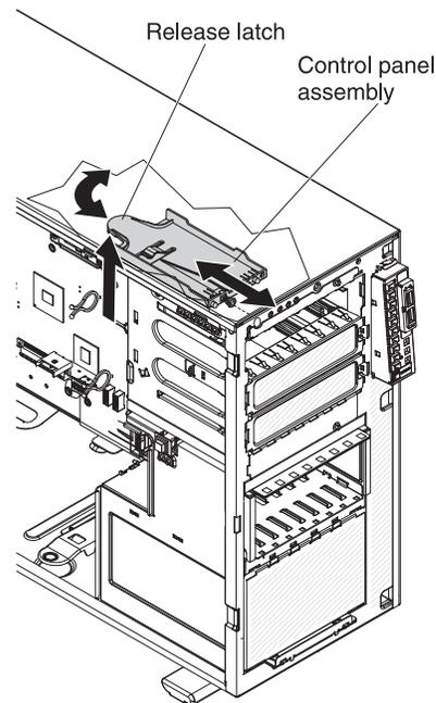
To remove the operator information panel assembly, complete the following steps:
