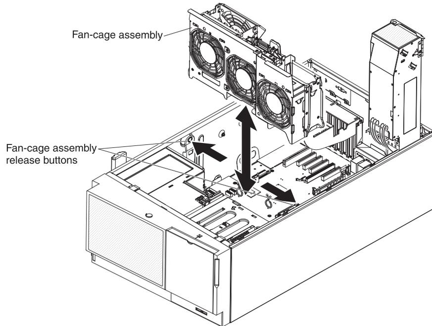
To install the fan cage assembly, complete the following steps.
