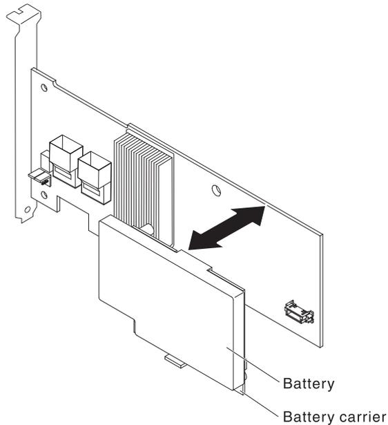
7. Insert the screws to secure the ServerRAID adapter battery in place.
