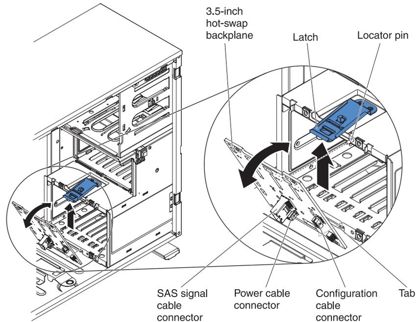
3. Reconnect the power, configuration, and signal cables to the 3.5-inch hard disk drive backplane. For more information, see *Internal cable routing and connectors*.
