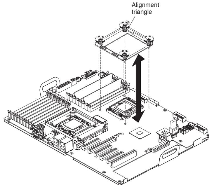
To remove a heat-sink retention module, complete the following steps:
