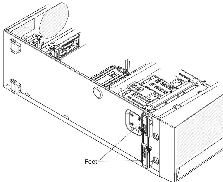
3. Reinstall the feet in the opposite location, with the tab on the feet extending beyond the edge of the server.
