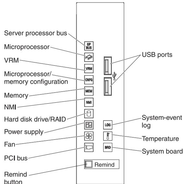
The following table lists the light path diagnostics LEDs, the problems that they indicate, and actions to solve the problems.
