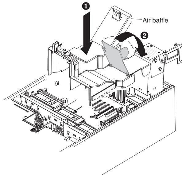
To install the air baffle, complete the following steps:
