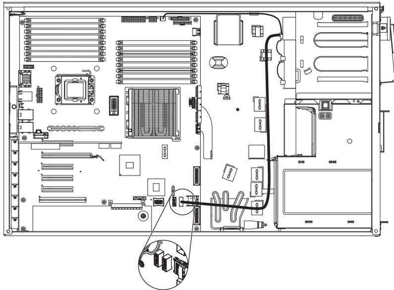
The following illustration shows the internal power cable routing and the connectors from the UltraSlim DVD drive to the system board.
