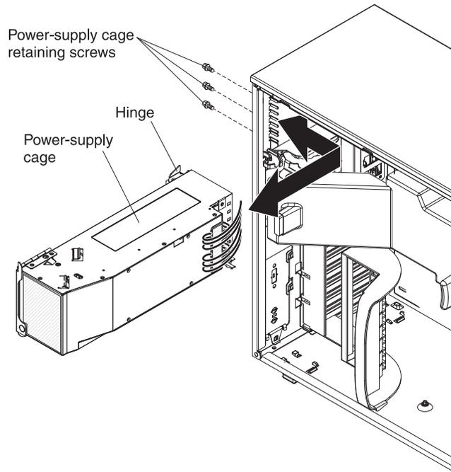
To remove the power-supply cage, complete the following steps:
