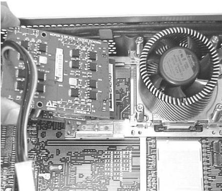
*Remove the Processor Power Pod*
