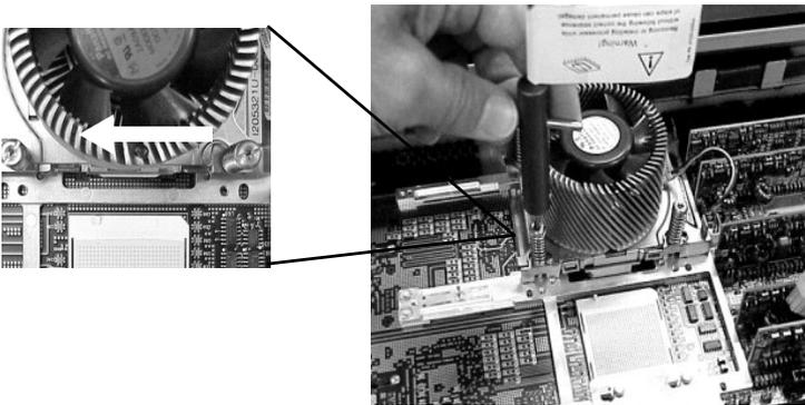
*Unscrew the Turbo Fan Heatsink Captive Screws*
