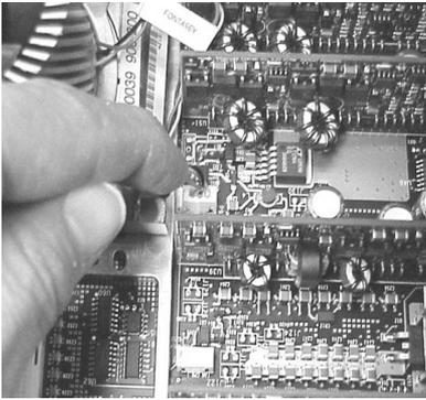
*Disconnect the Power Cable for the Processor Turbo Fan*
