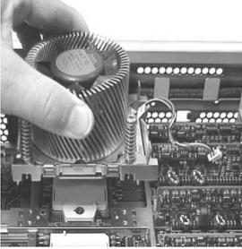
*Removing the Turbo Fan Heatsink and the Processor*
